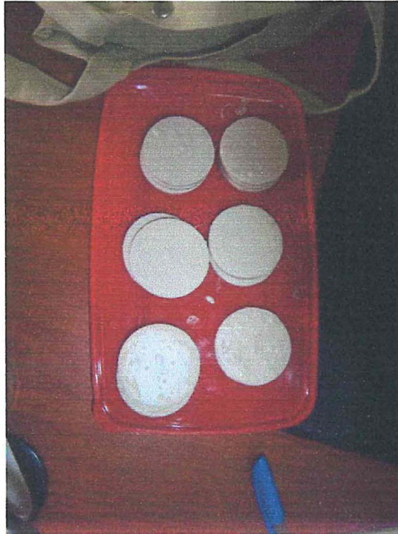
Figure 3.3: some of the fired samples formed by wet and dry pressing forming methods.
