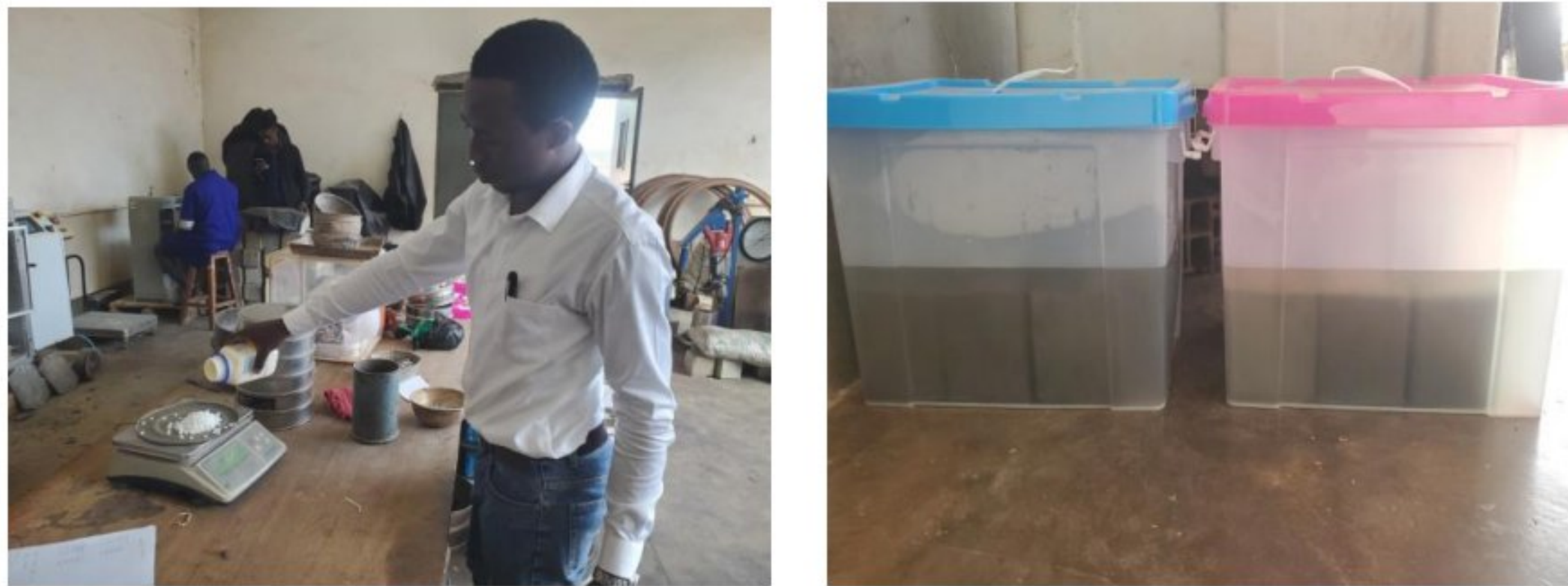
Figure 3.7 Pine needle and sisal fibre RC degradation (Durability test)
