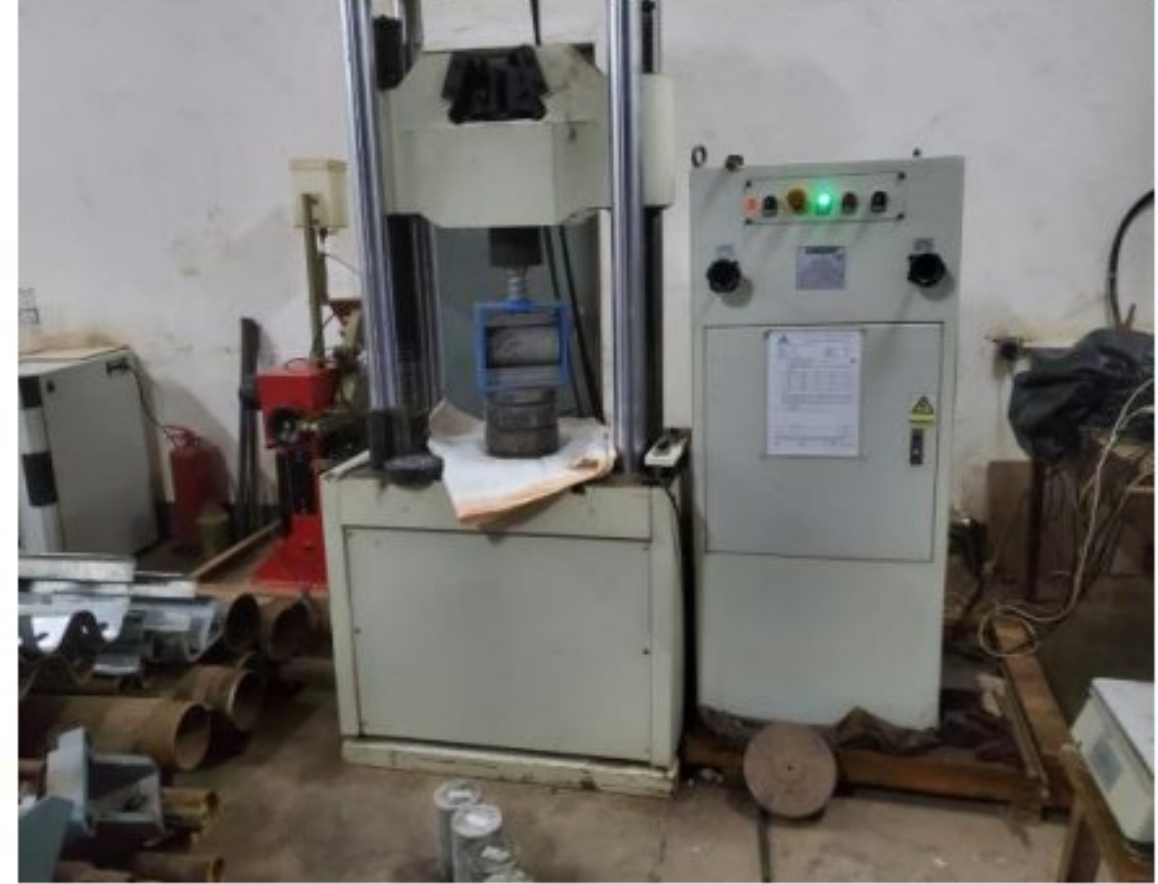
Figure 3.6 Sample Testing for compressive strength
