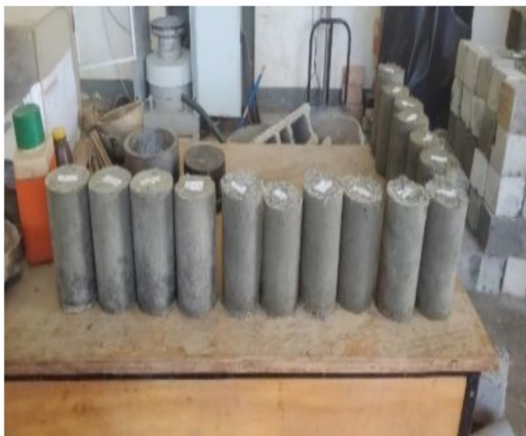
Plate A.11: Samples for split tensile strength test
