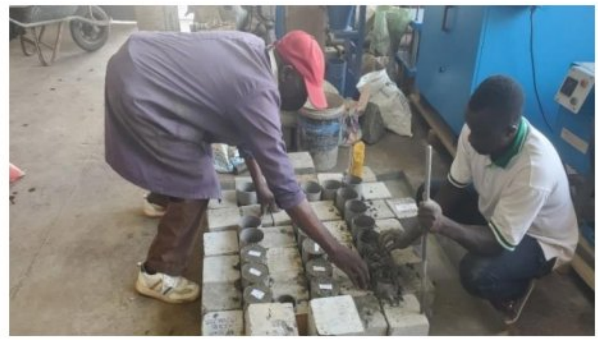
Plate A.10: Casting of split tensile strength samples
