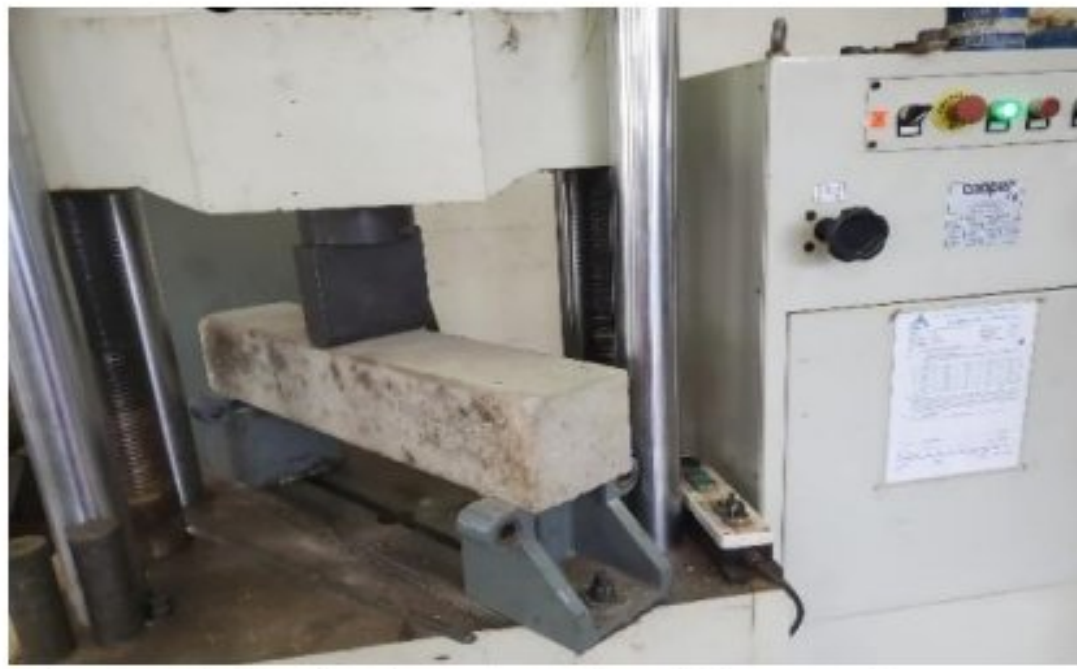
Plate A.7: A three point-flexural strength test
