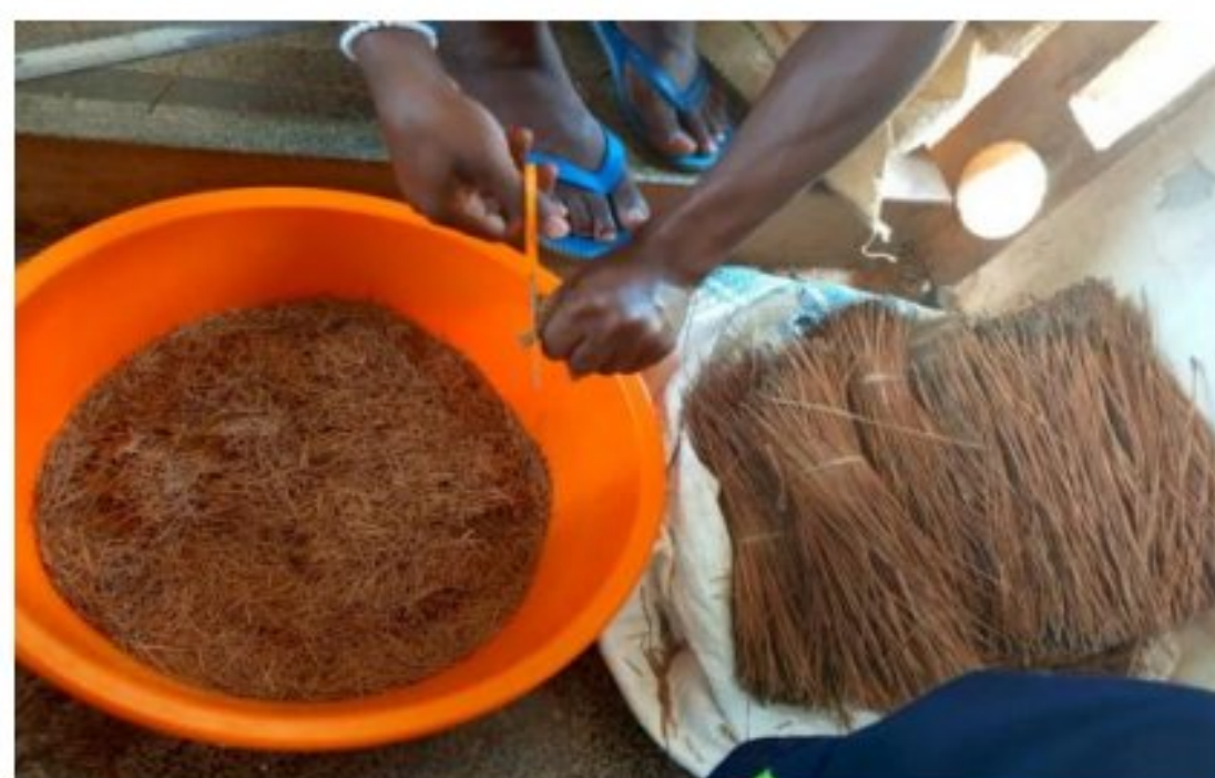
Plate A.6: Sorting and sizing of pine needle fibres
