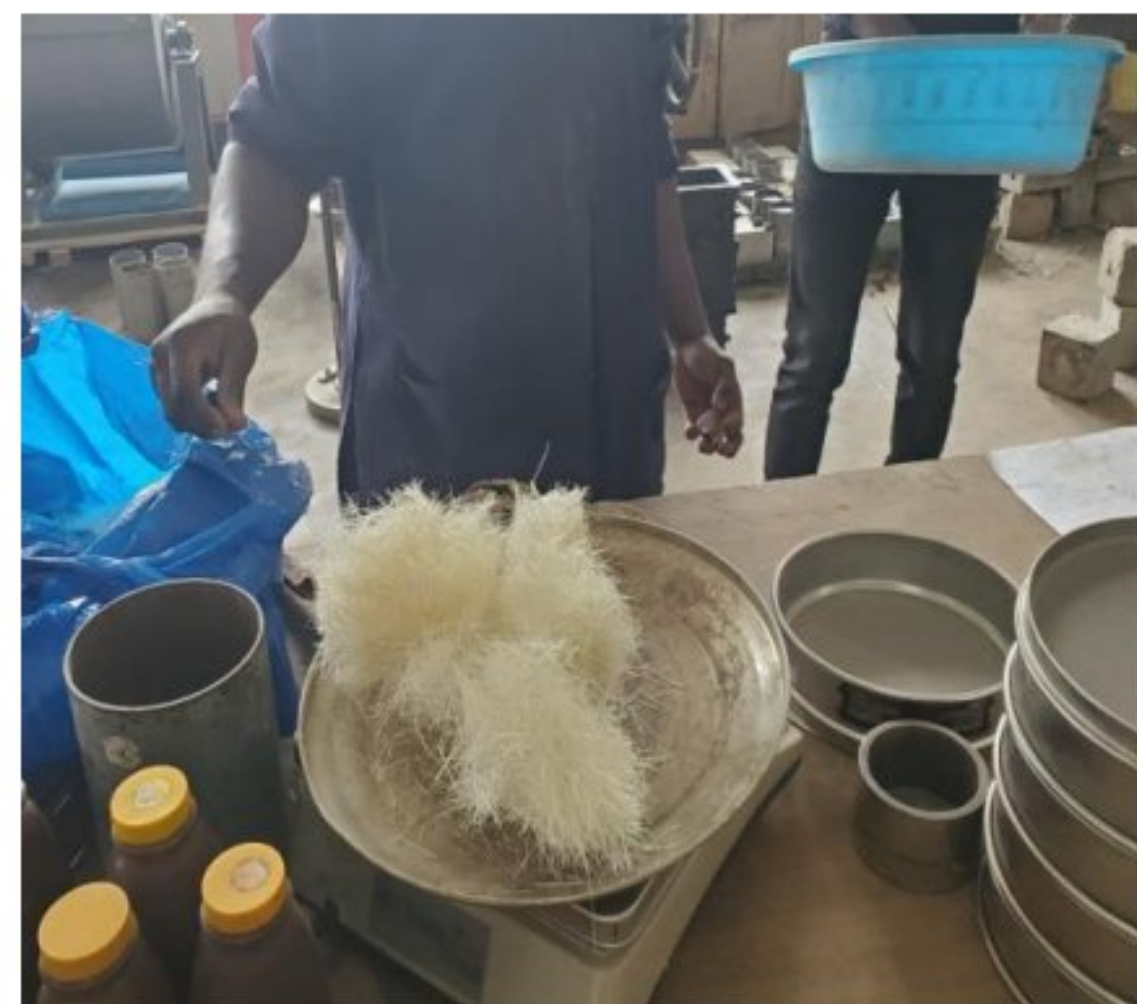
Figure 3.2 The process of weighing sisal fibres prior to its final preparation for incorporation into concrete
