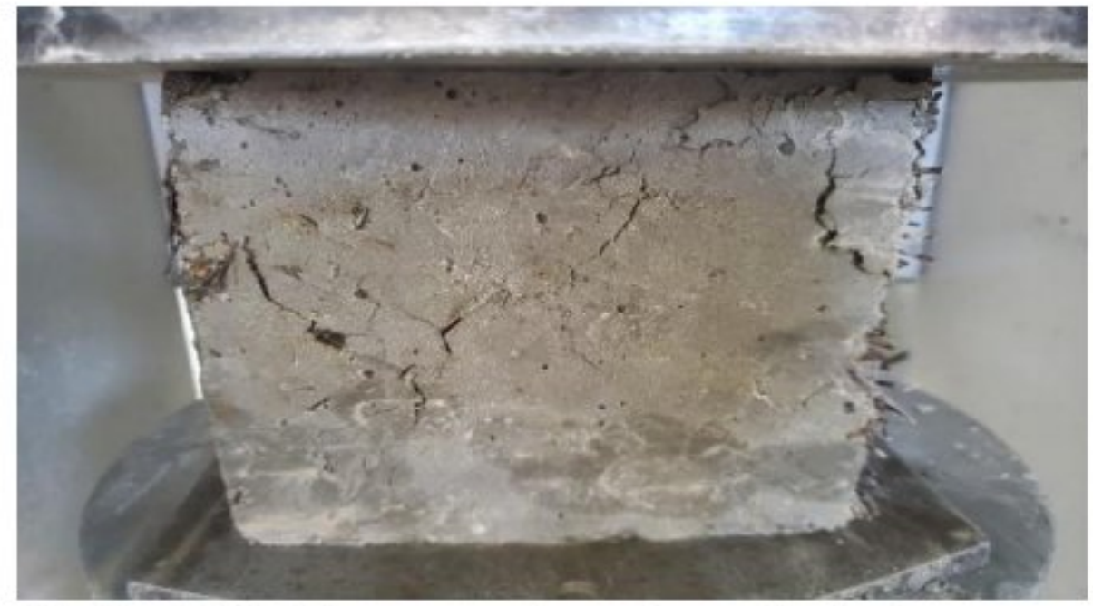
Plate A.8: Compressive strength test
