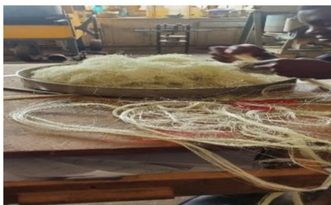
Plate A.5: Sorting and sizing of sisal fibres
