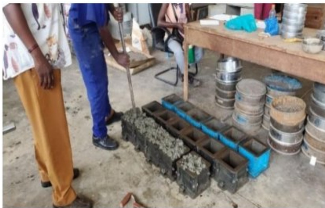
Plate A.9: Casting of compressive strength samples
