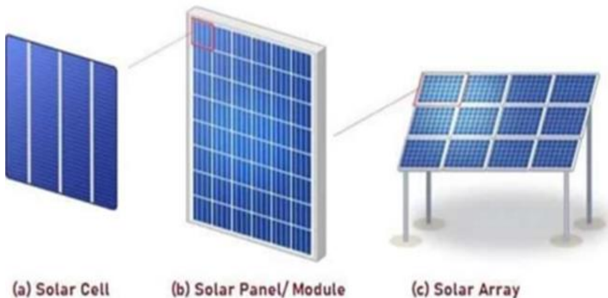
Figure 2.1: Illustration of (a) a solar cell (b) solar panel/module and (c) solar array. Reproduced with permission (Khaled et al., 2020).
