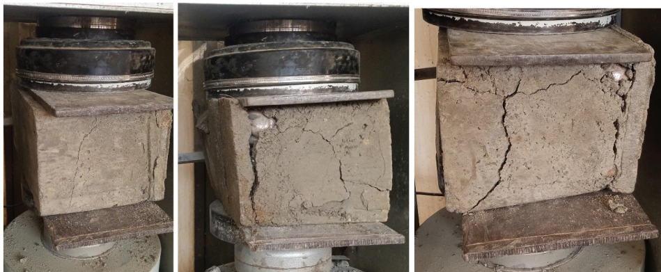
Figure 17. EBB block failure (left), PSB block failure (centre), SDB block failure (right).
