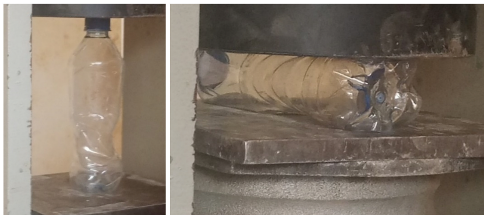
Figure 10. Buckling an empty plastic bottle in the vertical orientation (left), flattening of an empty plastic bottle in the horizontal orientation (right).
