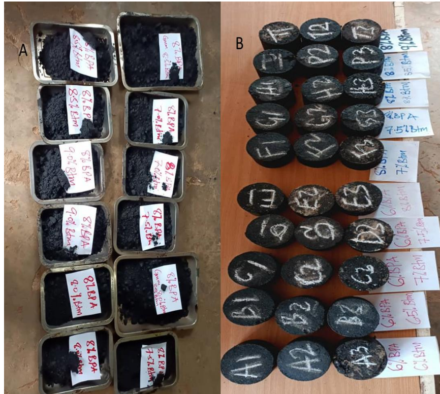
Figure 3.10: (A) 6 % BPA mixed samples and (B) Compacted samples of 6% and 8 % BPA
