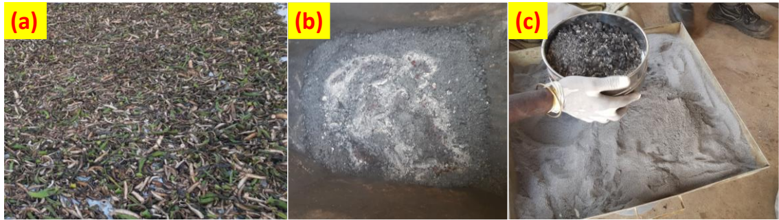
Figure 3.4: (a) Drying of banana peels, (b) Banana peels during incineration in the chamber, and (c) Sieving of cooled BPA using 0.075 mm diameter sieve
