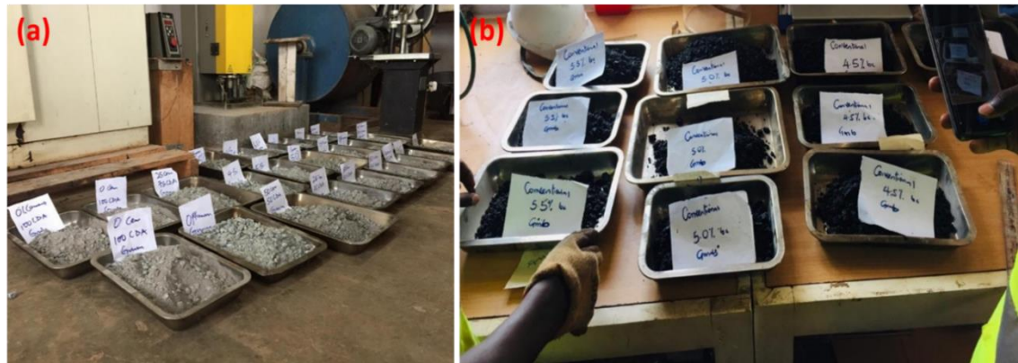
Figure 3.8: (a) Dry aggregate and cement mix and (b) Aggregate, cement and bitumen mixed materials
