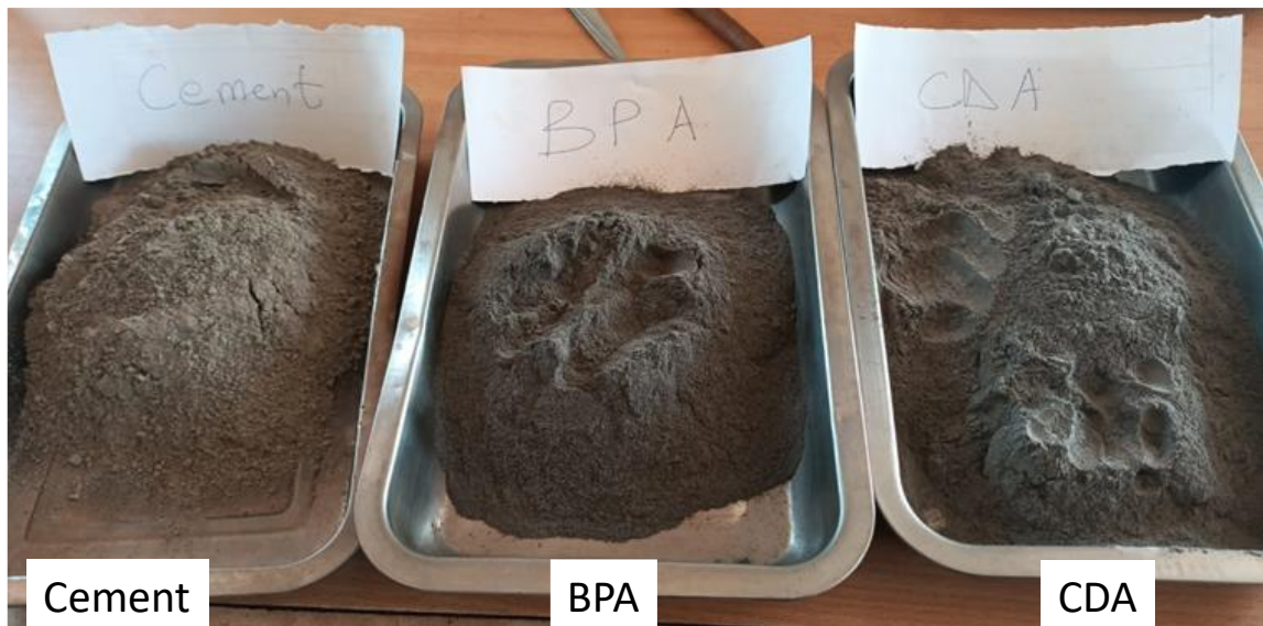
Figure 3.6: Filler materials (Cement, Banana peels ash (BPA) and Cow dung ash (CDA))
