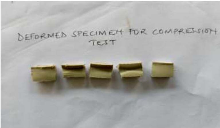
Figure 4- 9. Deformed specimen after a compression test
