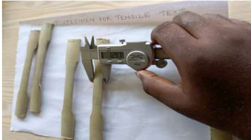
Figure 3- 8. Tensile test specimen cut out from the PPH pipe
