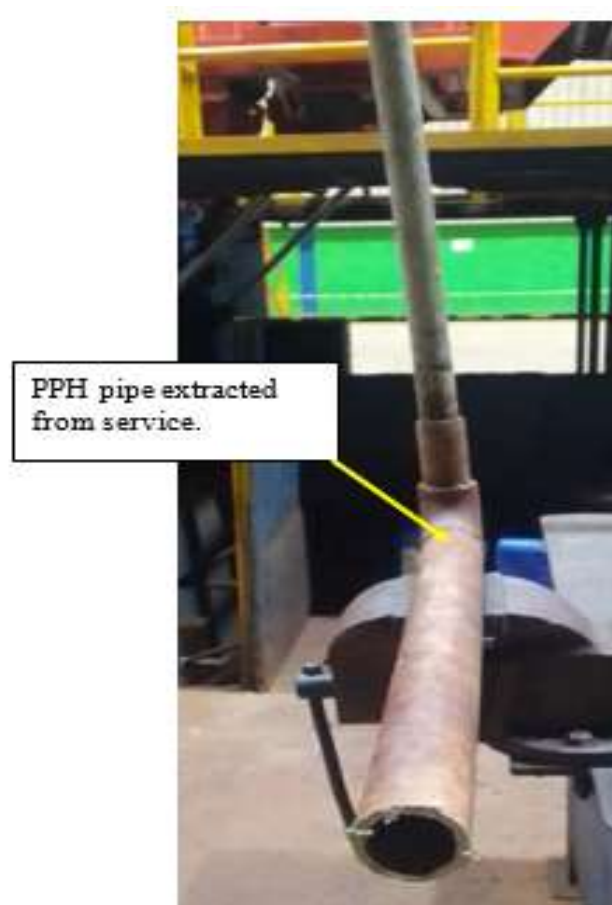
Figure 3-6. PPH d63 DN50 SDR 33 pipe extracted from Service
