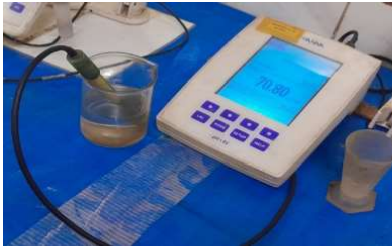
Figure 3- 3. Conductivity meter for Testing the Condensate
