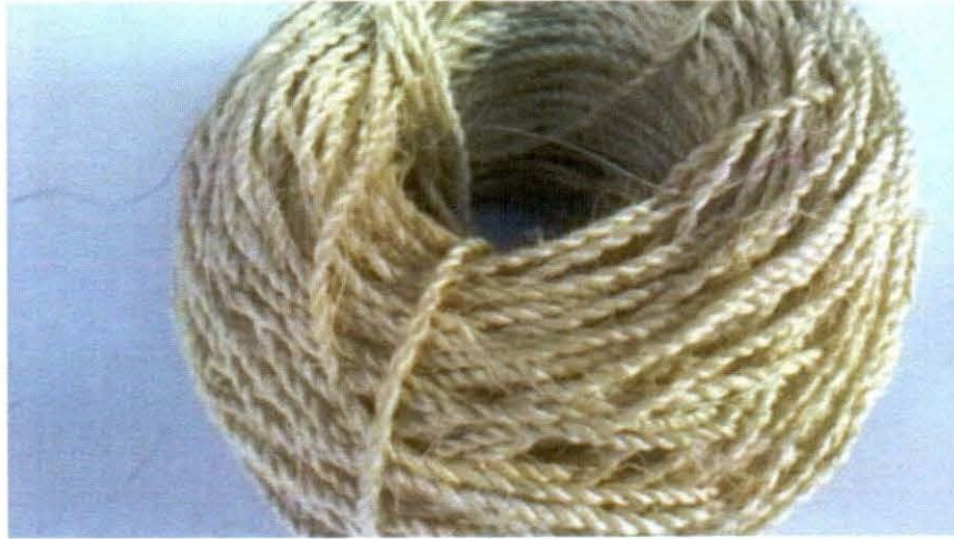
Fig a: Plain two ply sansevieria fibers Source: photo by the researcher (2017)
