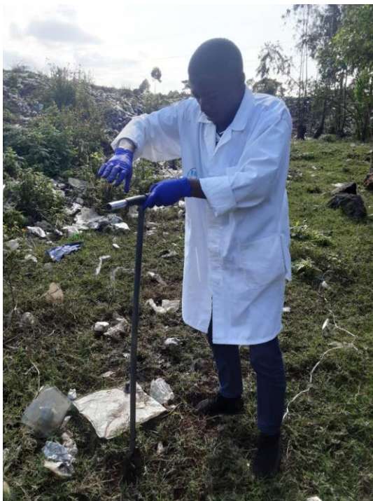
Usage of soil Auger for soil sampling in wet and dry seasons, and soil sample preparation respectively at the laboratory
