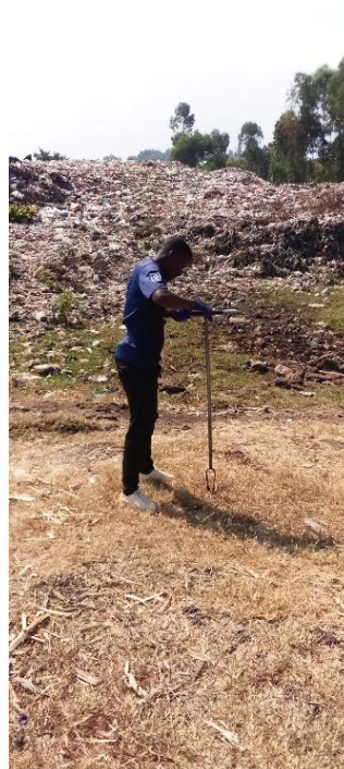
Usage of soil Auger for soil sampling in wet and dry seasons, and soil sample preparation respectively at the laboratory
