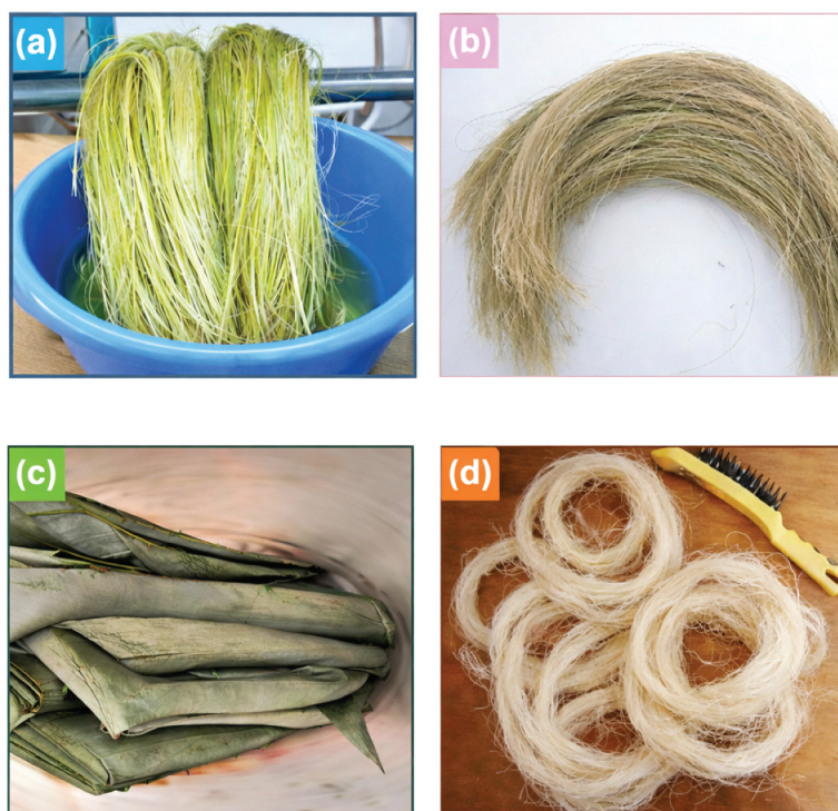
Figure 1. Sequential fiber extraction process: (a) Stipa tenacissima (Alfa) plant used as raw material; (b) Stipa tenacissima fibers after water retting, washing, and drying; (c) Agave americana plant used as raw material; (d) Agave americana fibers after water retting, washing, and drying.
