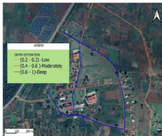
Figure 3. The Depth of a 1-inch Diameter Pipe
