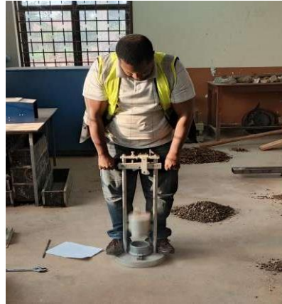
b. AIV test. Sieving is done after the test and the sample is weighed again
