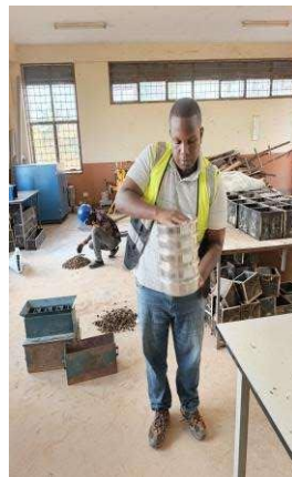
h. Shaking sample using stack of sieves
