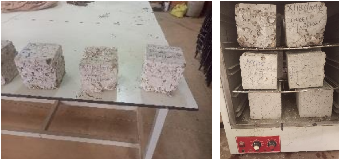
Figure 4- 25: Cracked concrete cubes
