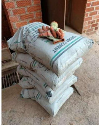
a. CEM II, 32.5N (Tororo) Cement used
