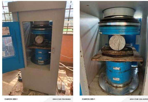
Figure A.6.15 : Splitting Tensile Strength Test being carried out
