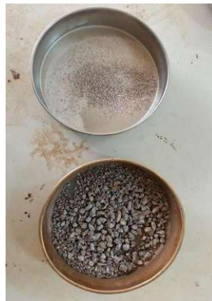
b. Sieving is done after the test and the sample is weighed again
