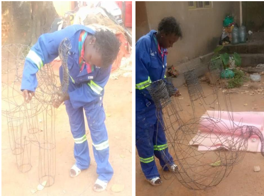
Figure 39; Rolling annealed binding wires on the amateur.
