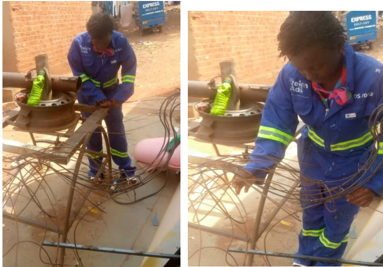
Figure 38; The researcher curving annealed binding wires to make rings using a bender.
