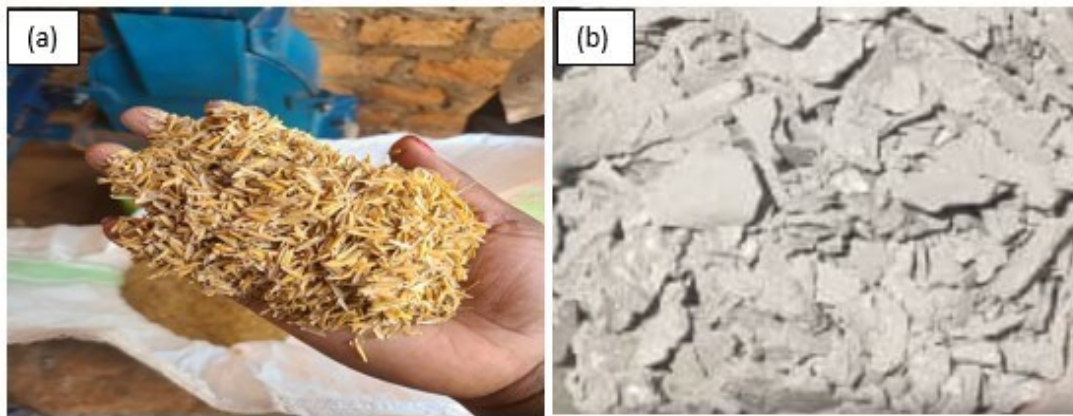
Figure 3. 2: (a) The rice husks used and (b) ball clay sourced from Ntawo deposit.
