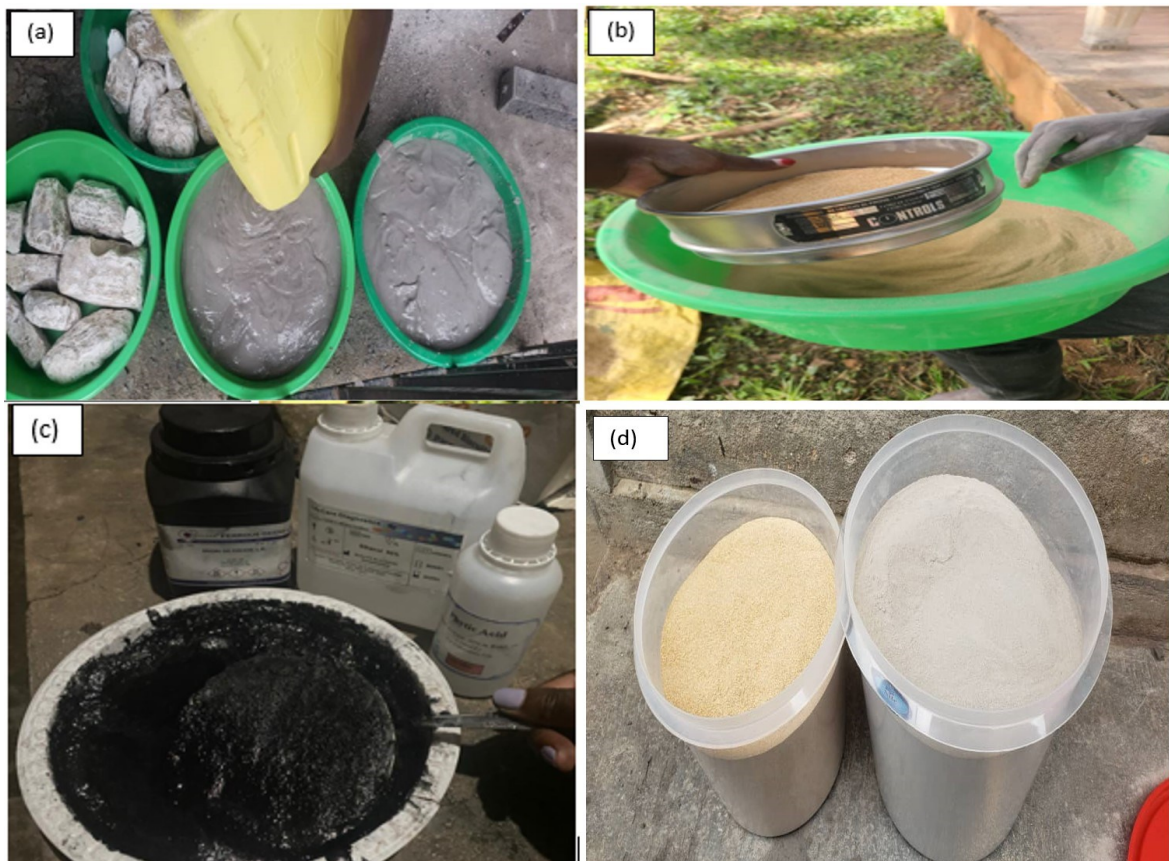
Figure 3. 3: (a) Preparation of ball clay, (b) sieving of rice husks powder to obtain fine powder, (c) colloidal solution of iron oxide, and (d) prepared fine powders of rice husks and clay.
