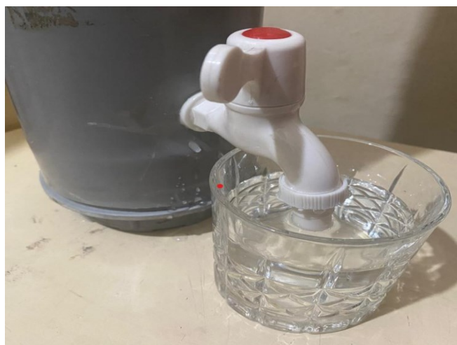
Figure 3.8: Collection of influent water using the PoU filter.
