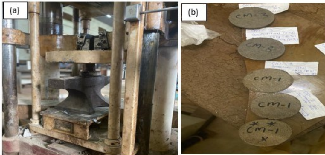
Figure 3.4: (a) Pressing machine used for membrane pressing and (b) the green body of the prepared disks.
