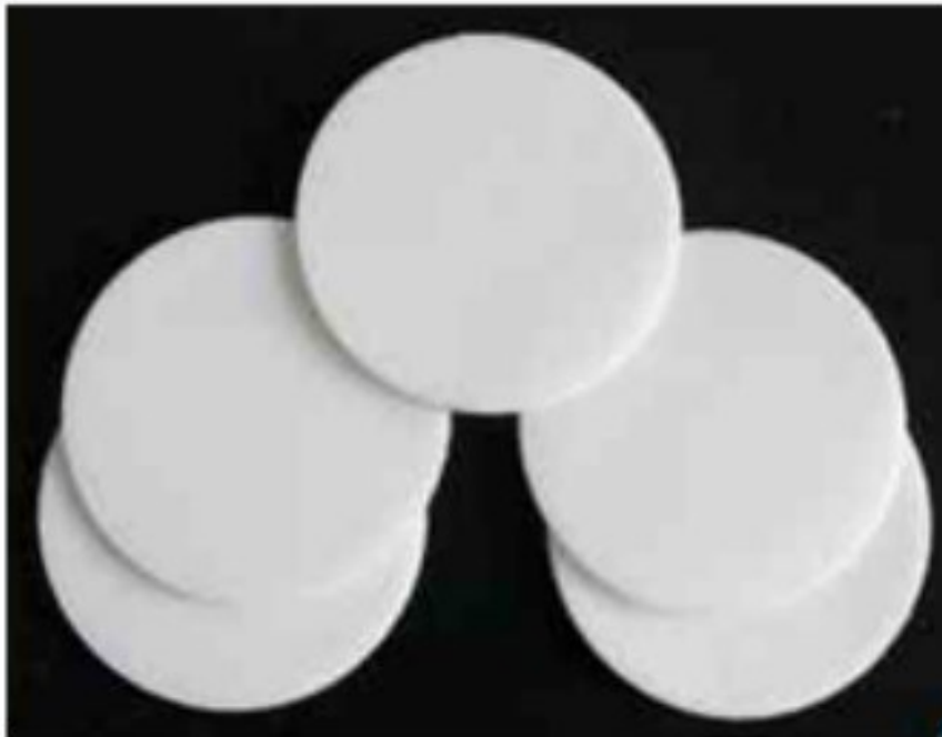
Figure 2.1: Plate ceramic membranes (Amin et al., 2016)
