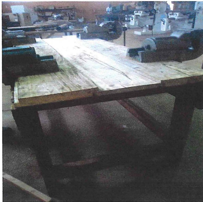
Fig. 23 Refurbished bench with vices firmly fixed.
