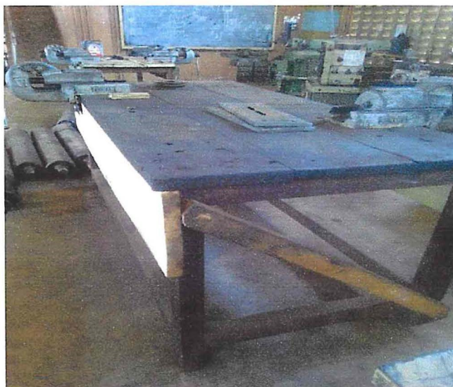
Fig. 27 Refurbished bench with two vices fixed
