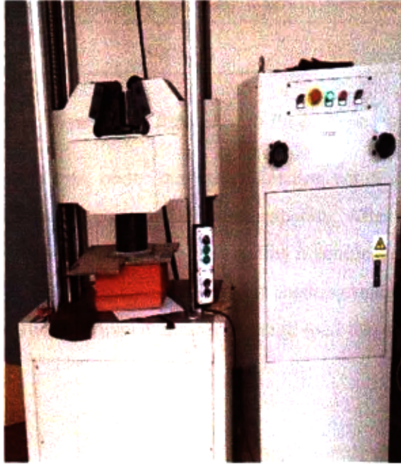
Plate 3.1: Crushing of Hollow Block Perpendicular to Holes
