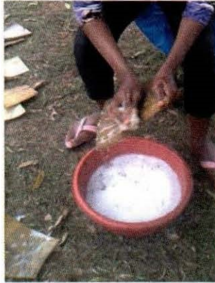
Figure 4.77: Washing the flattened pieces of the cow horn. Photo by researcher - courtesy of Cow horn workshop – Nakawa, Kampala
