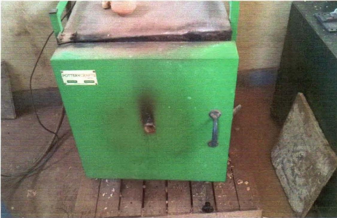
Figure 3. 4: Picture of an Electric kiln used for firing the Clay Samples
