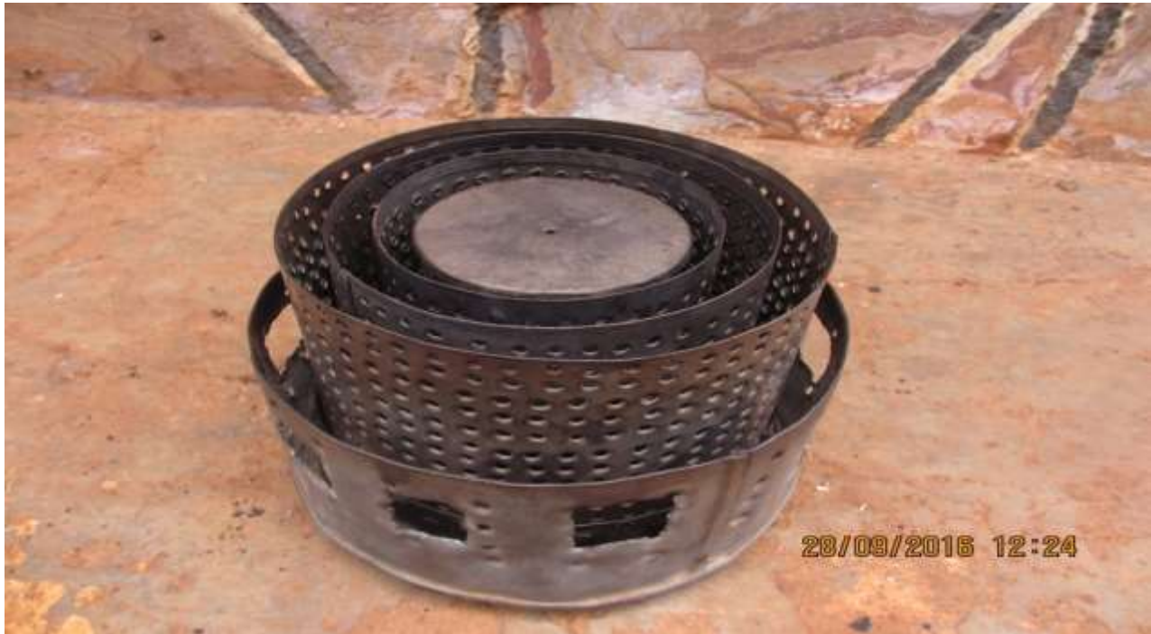
Figure 3.16: Picture of the charcoal holder, fuel holder, flame holder assembled together.
