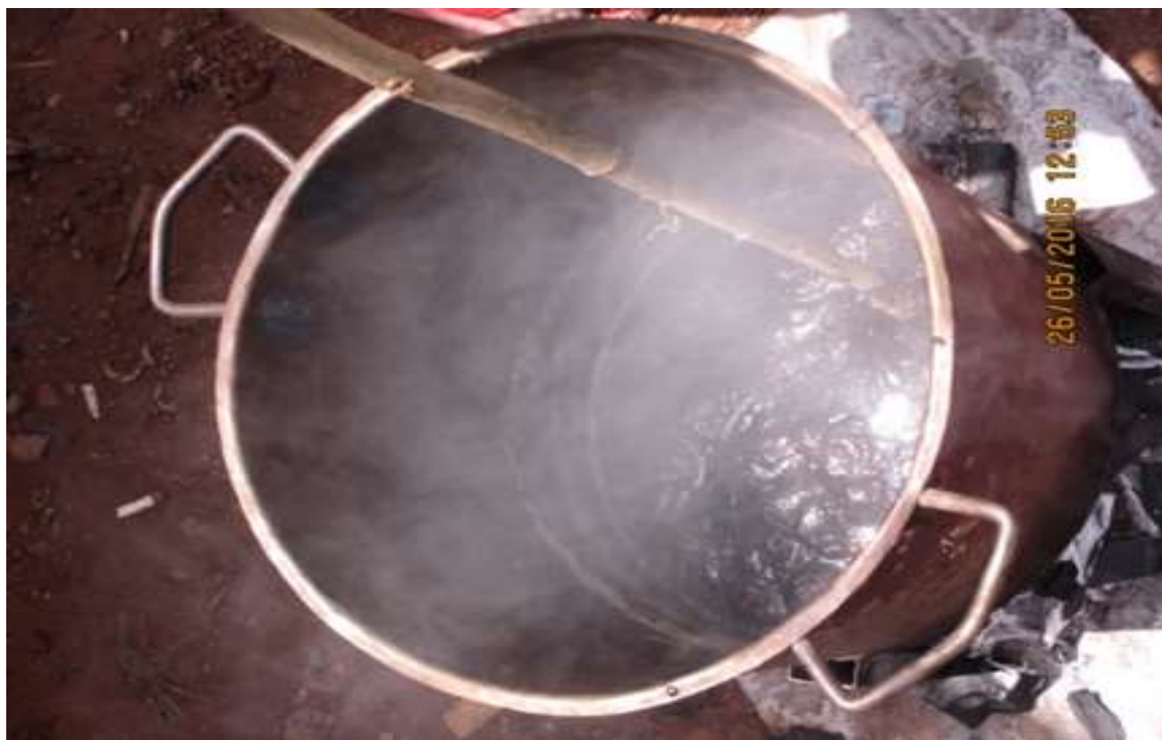
Figure 3.3: Picture of molten plastic in the boiler.
