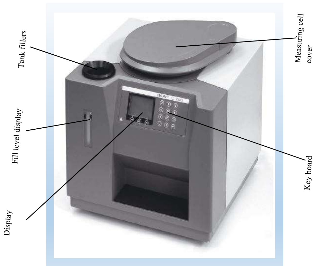
Figure 3.17: Features of the bomb calorimeter C 200 Model.
