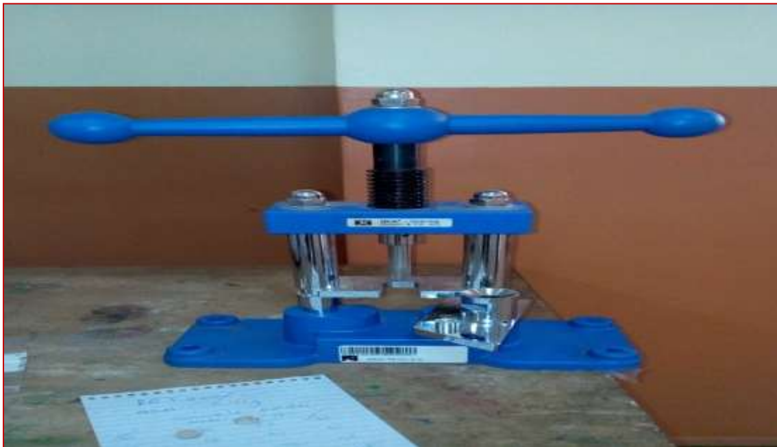
Figure 3.6: Picture of the pellet making machine.
