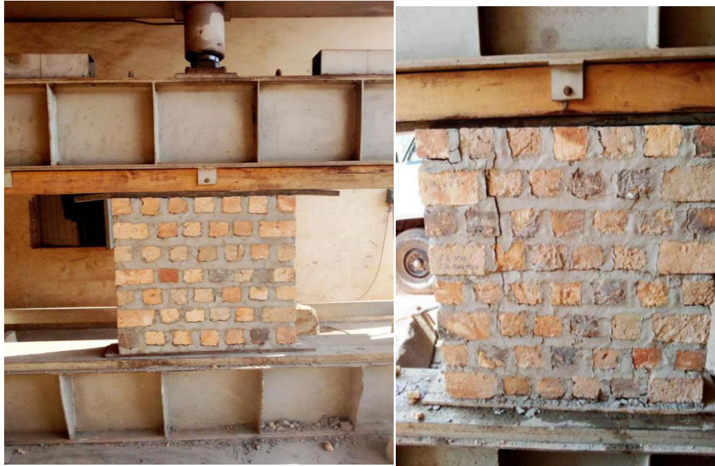
Figure 4. 12: Wall structure (1000 x 1000) mm tested and failure of the walls)
