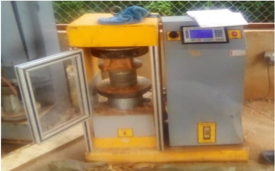
Figure 3. 1: Compression testing of bricks and mortar
