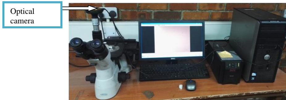
Figure 3.13 Metallurgical Microscopes (MUK, 2018)
