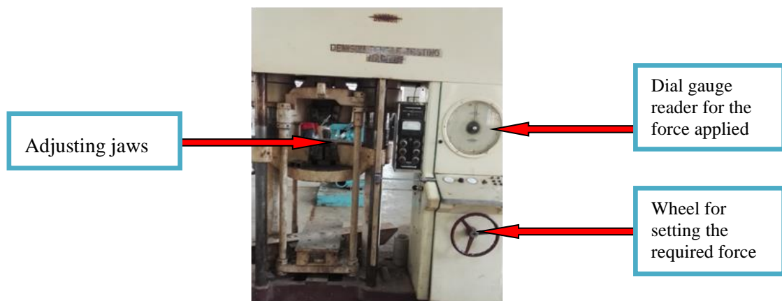
Figure 3.1 Universal Tensile Testing machine (KYU, 2018)
