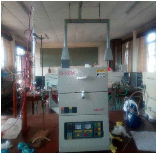
c) The tubular furnace pyrolyzer (center), the vacuum pump (Right) and the U-tube manometer (left).
