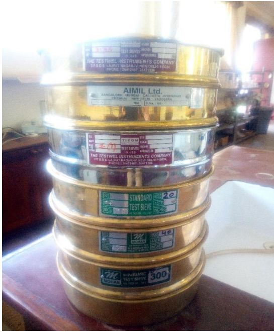
a) Standard test sieves used for Particle size screening
