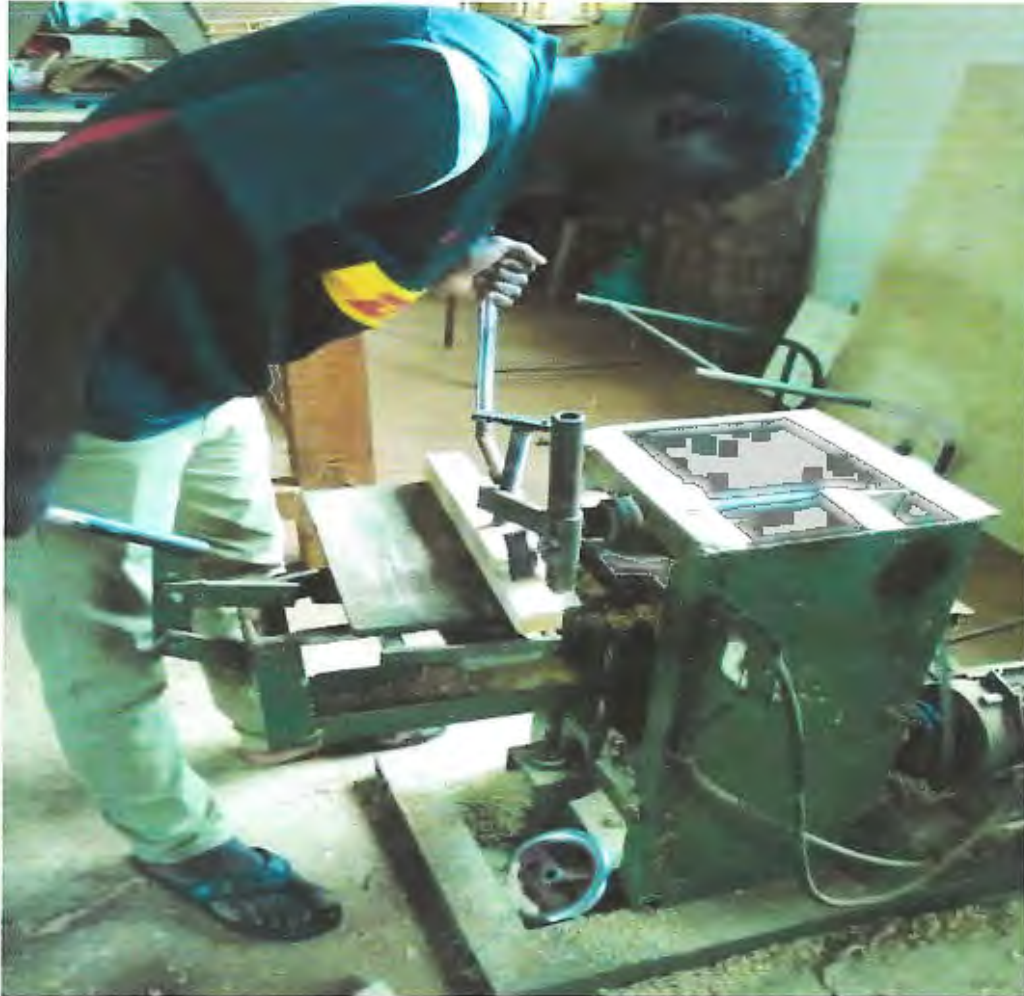
Fig.22: Learner Morticing Timber Piece Members for Construction of the Church Pew ( Source: Primary Data, 2018 )
