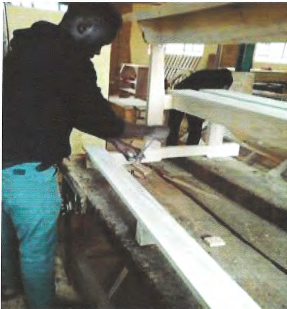
Fig.26: Preparing and Fixing Kneelers onto Main Furniture Piece, Process Continues ( Source: Primary Data 2018 )
