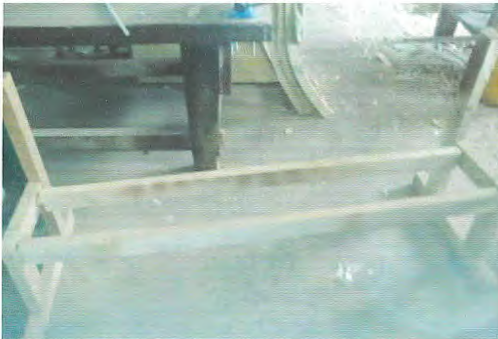
Fig.38: Church-Pew piece members were not cleaned, fixed and sandpapered ( Source: Primary Data 2018 )
