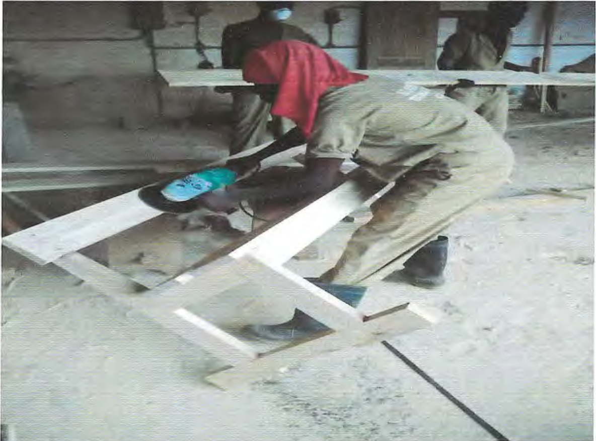
Fig.16: Implementation of Smooth Wood Surface-Finish Strategy by Application of Angle Grinder Machine. (Source: Primary Data,2018)
