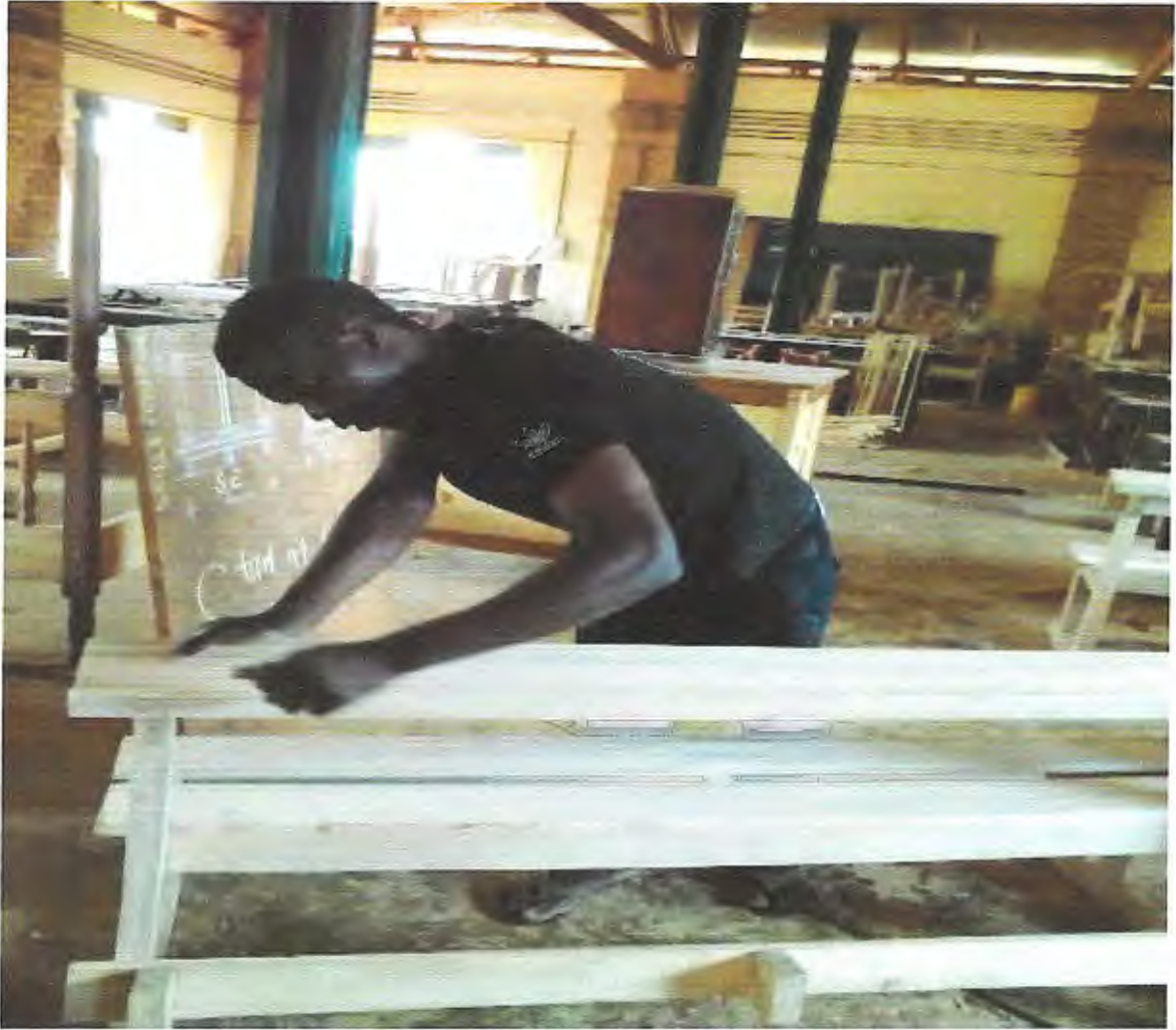
Fig.34: Trainee Giving His Church-Pew a Last Sandpapering- Finish, Using a Waterproof Sand Paper (Source: Primary Data 2018)
