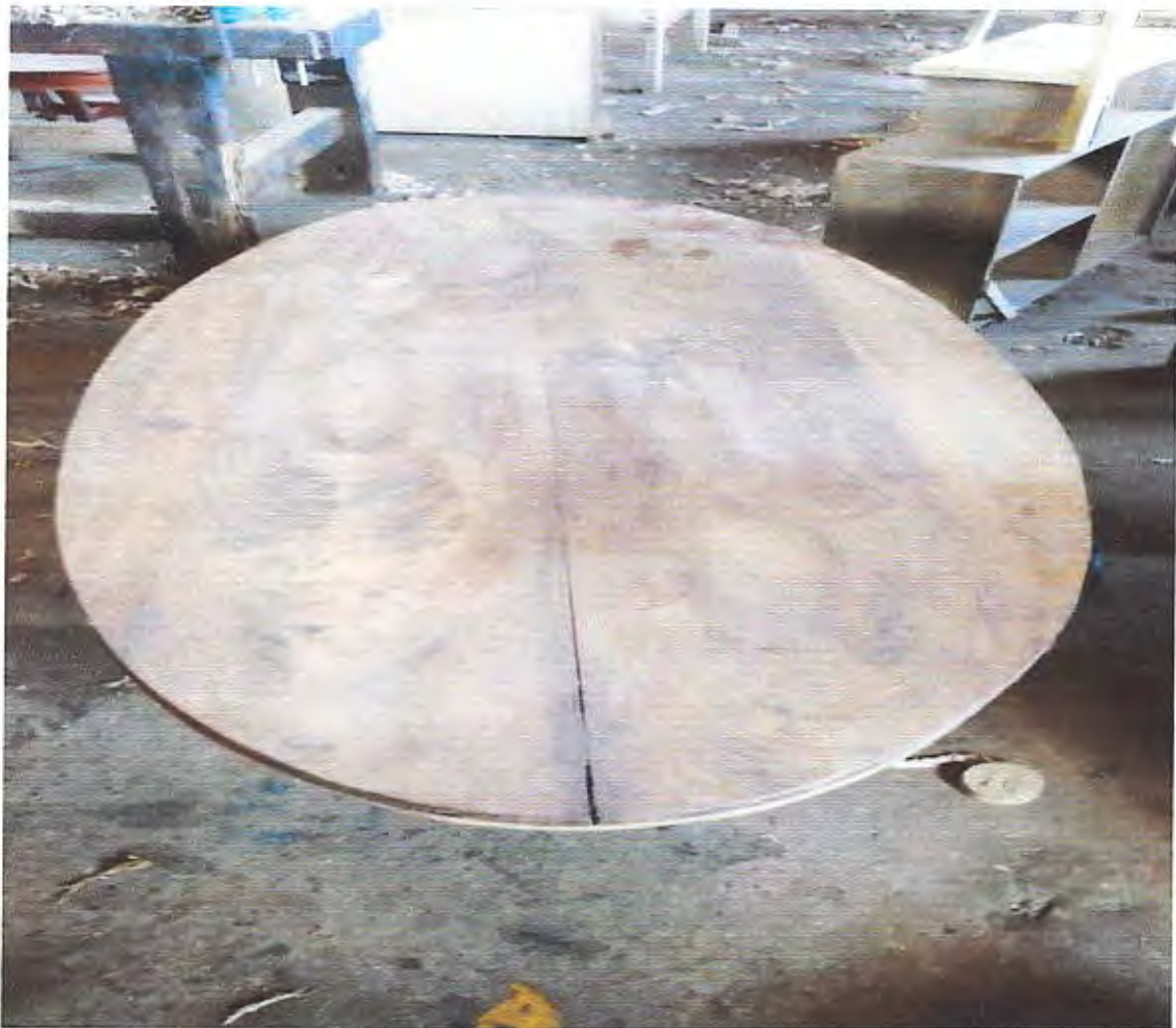
Fig.6: Showing Open Joints in Finished Furniture Due to Using Wet Timber. (Source: Primary Data 2018 )
