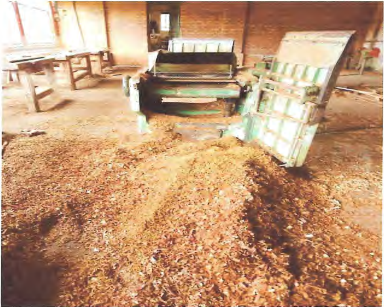
Fig. 2: Thicknessing Machine Used to Dress(Plain) Timber; DWWT (Source: Primary Data 2018 )
