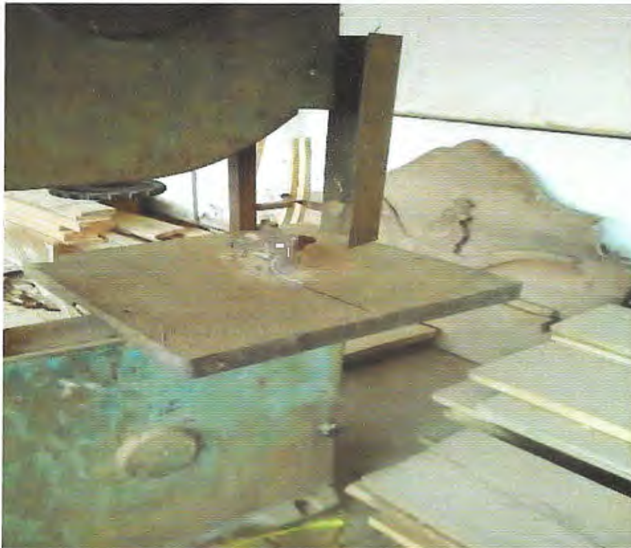
Fig.23: A Band Saw Machine Lying Idle, Could Not Cut Curves in Some Timber Piece Component to A Church Pew, Lacked A Blade (Source: Primary Data 2018 ).
