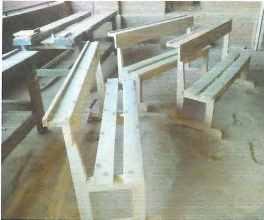
Fig. 37: Furniture Pieces Still Lacked Some Components, Was Not Cleaned, Fixed and Sandpapered, Could Not Be Varnished ( Source: Primary Data 2018 )
