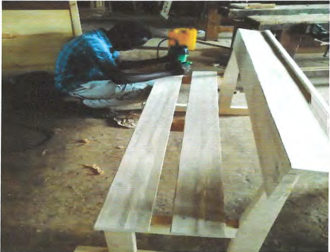
Fig. 33: Trainee Applying a Router Plane On His Work for Molding Formation, For Skill's Improvement (Source: Primary Data 2018 )
