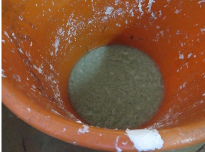
Figure 12: Showing Pulp soaked Sodium hydroxide
