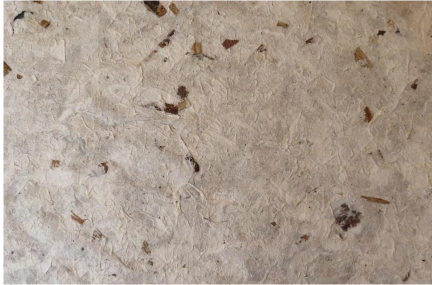
Figure 24: Surface produced from banana fibres, waste cotton offcuts and banana fibre offcuts
