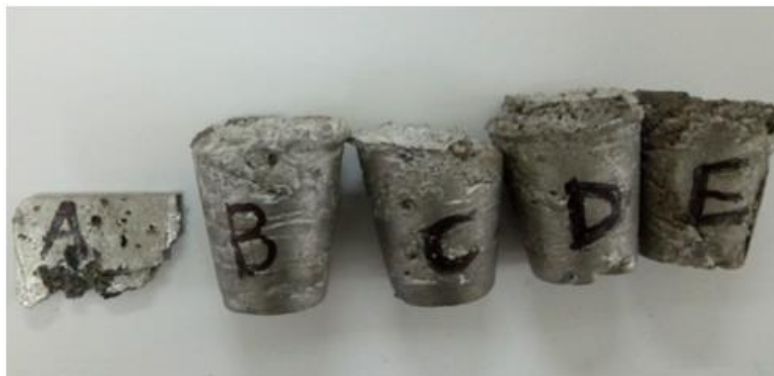
FIG. 3- 3 Specimens obtained from top Al-Zn dross samples extracted at different intervals.
