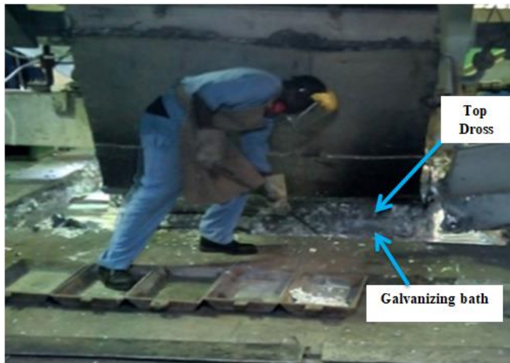
FIG. 3- 1 Harvesting of top Al-Zn dross during an ongoing galvanizing process
