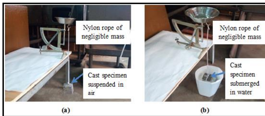
FIG. 3- 14 Measurement of the mass of the top Al-Zn dross/ portland pozzolana cement slabs
