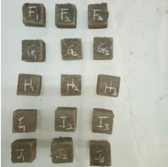
FIG. 3- 12 Concrete specimens used for determination of density and porosity
