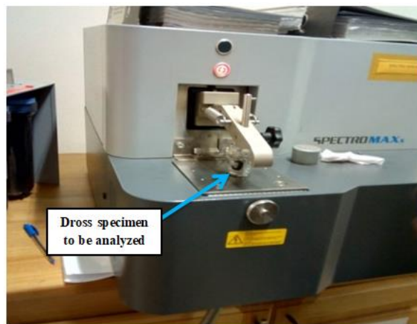
FIG. 3- 5 Specimen mounted on the spark absorption spectrometer for analysis
