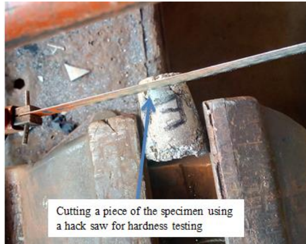
FIG. 3- 6 Cutting the top Al-Zn Dross specimen to size using a hack saw
