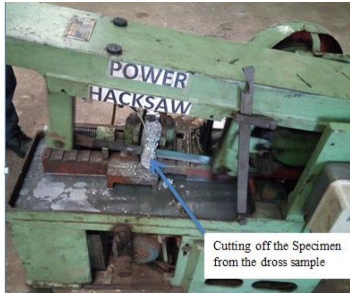
FIG. 3- 2 Cutting the top Al-Zn dross samples with a power saw
