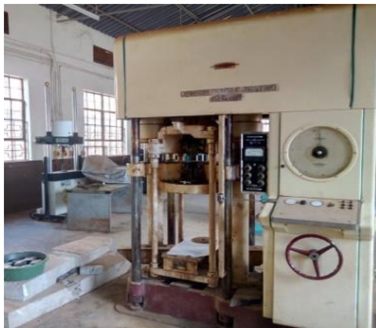
FIG. 3- 20 Denison compressional testing machine, model T.42B4, capacity 500KN
