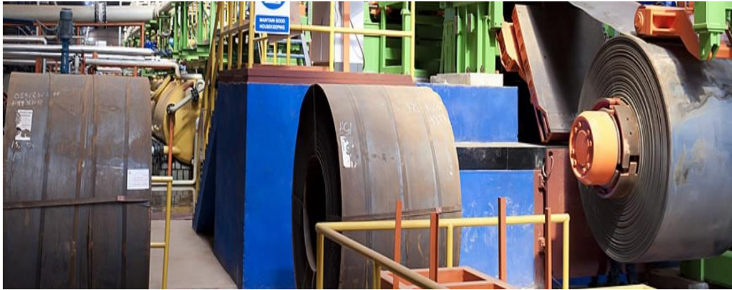
Figure B-1 : The coiled rolls ready to be pickled (on site pictures)
