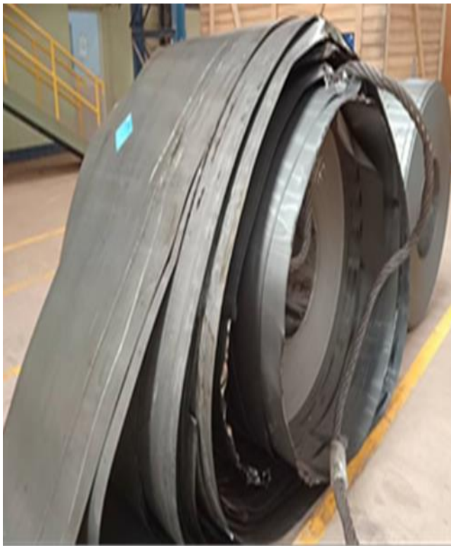
Figure B-6 : Damaged roll of coiled sheet (edges) (on site pictures)
