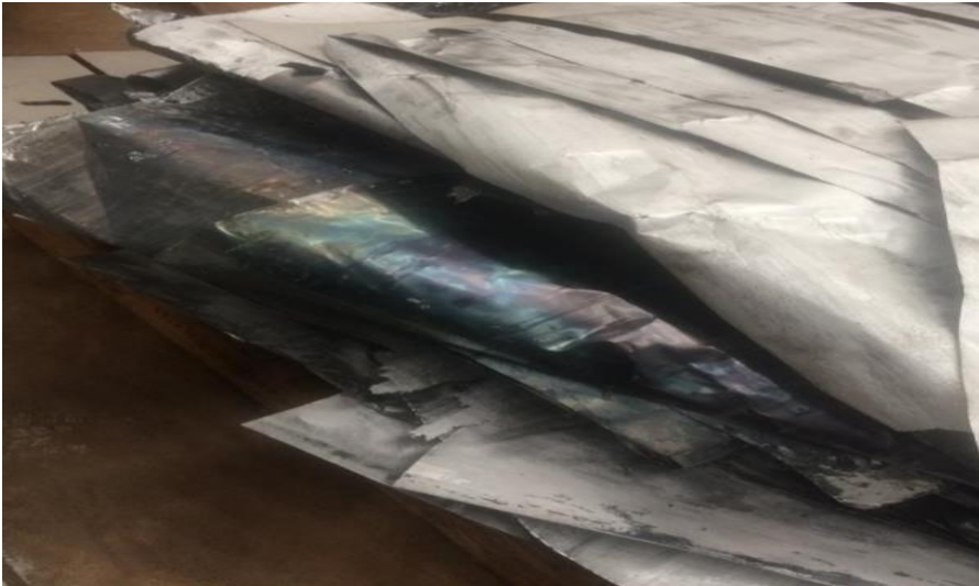
Figure B-9 : Damaged sheet (burnt) (on site pictures)
