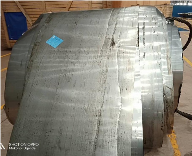
Figure B-7 : collapsed roll of coiled sheet (on site pictures)
