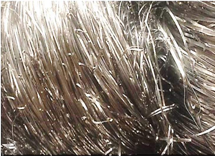
Figure B-8 : Coiled cut strips of sheet (rejects) (on site pictures)
