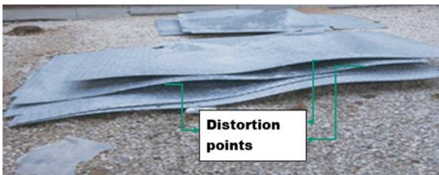
Figure 4-9 : Distorted sheets (on site pictures)
