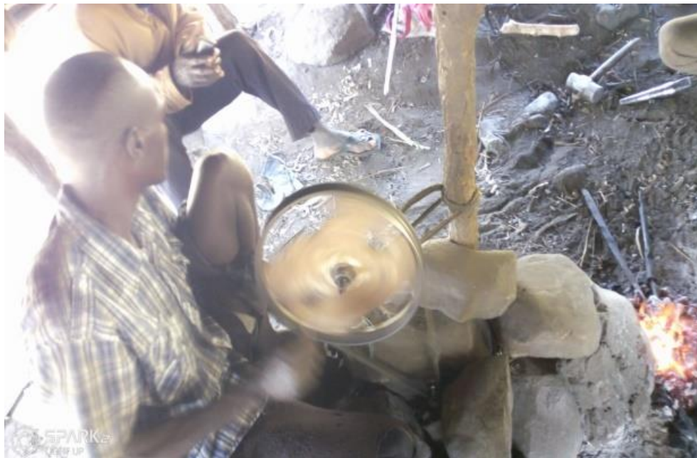
Figure 4.6: The smelter working the bellows (lor buk).
