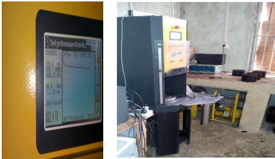
Figure 3.21: Gyratory Compactor and its recordation system
