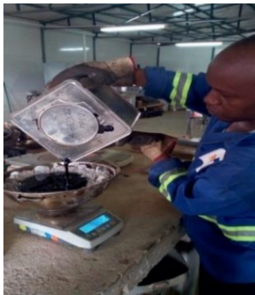
(a) Weighing bitumen
