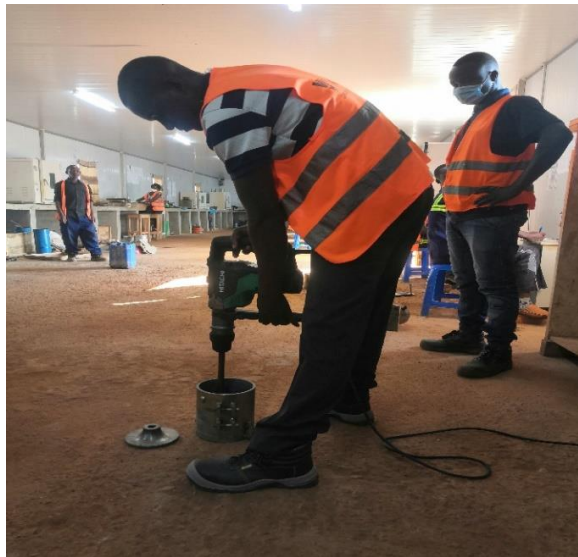
Figure 3.20: Electrically operated vibrating hammer compaction
