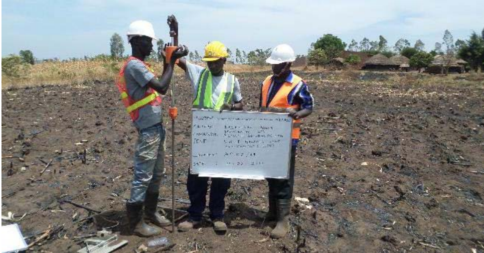
Figure 3.2: Dynamic Probing Light (DPL) test in the field
