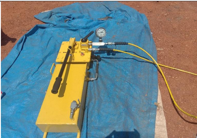
Hydraulic Pressure Pump and gauge system
