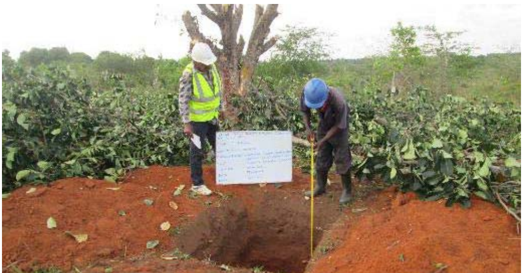
Figure 3.1: Typical excavated trial pits
