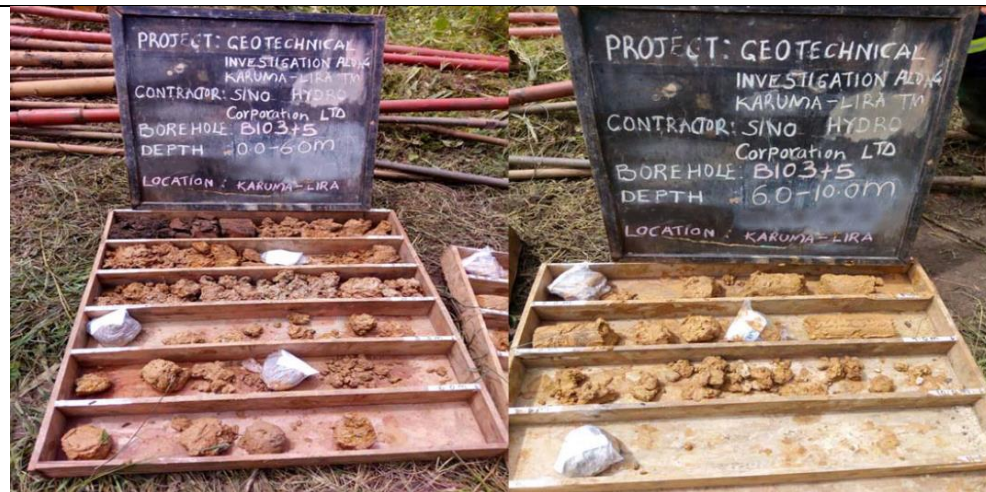
Sample boxes for KL 30 (B103+5) from 0.00-10.00 m
