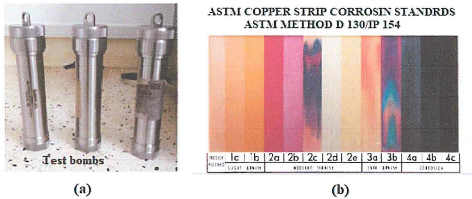
Figure 3.6: (a) Test bombs, and (b) ASTM copper strip corrosion standards
