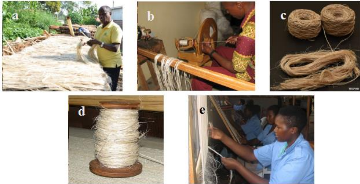
Figure 10: Production of banana fiber yarn that is suitable for weaving into fabric at Texfad
