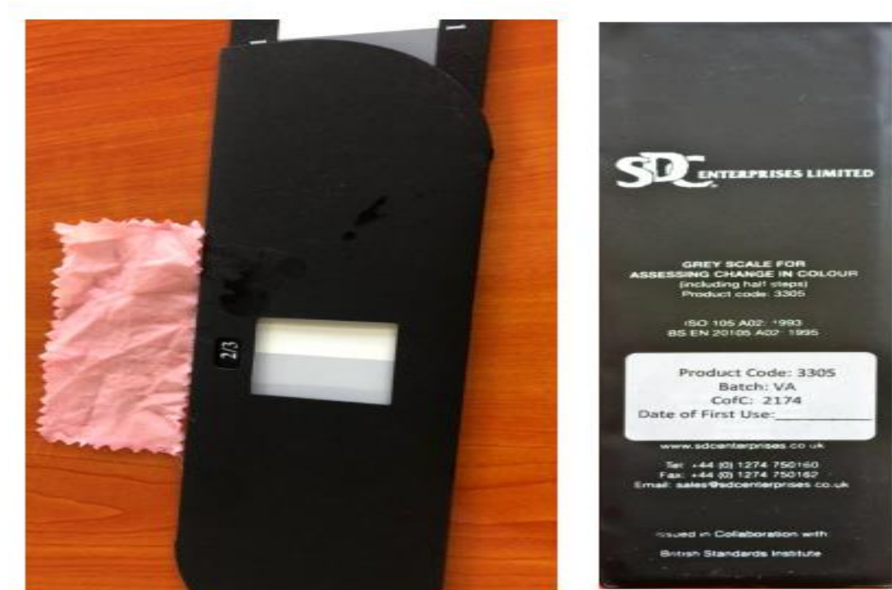
Figure 34: Grey scales for assessing the change in color during the color fastness testing
