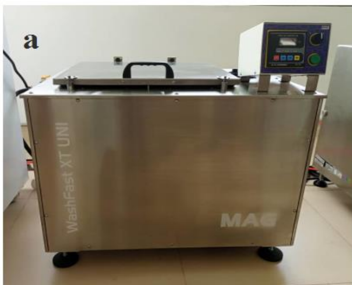
Figure 24: (a) a laundrometer machine used to test the wash fastness of textiles and (b) a sample of Cyperus papyrus woven product.
