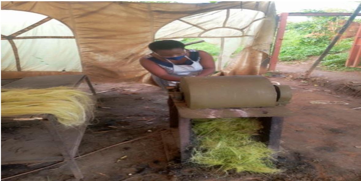
Figure 19: Photo showing the machine extraction process of Cyperus papyrus fibers.
