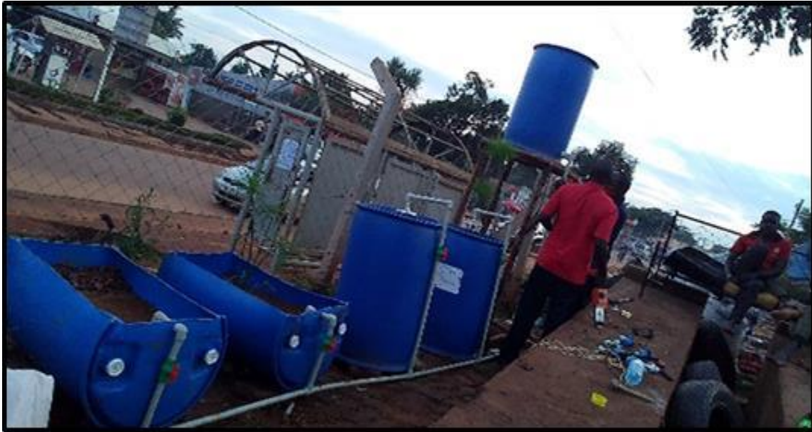
Figure 3-6 : Waste water treatment systems layout (Right to Left: overhead tank, Vertical flow drum (planted and unplanted) and Horizontal flow drum (planted and unplanted).
