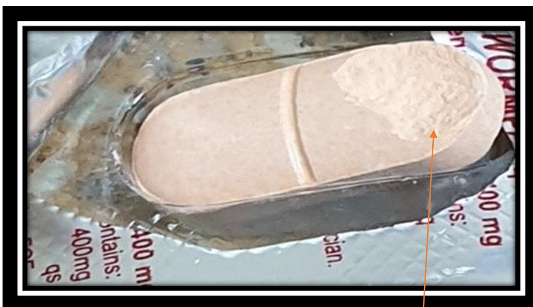
Chipped tablet observed during visual inspection
