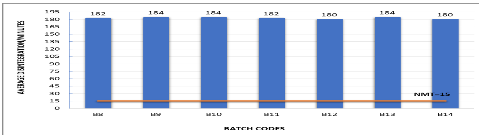
Fig 4. 4: A bar graph showing the batches of Albendazole chewable tablets that failed the Disintegration test
