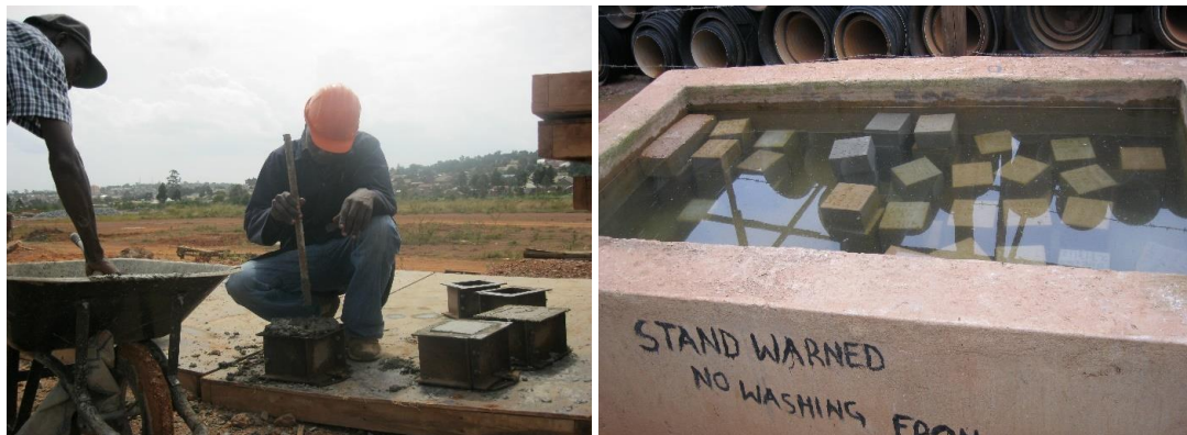
Figure 3.7: Preparation and curing of concrete cubes for compressive strength test.
