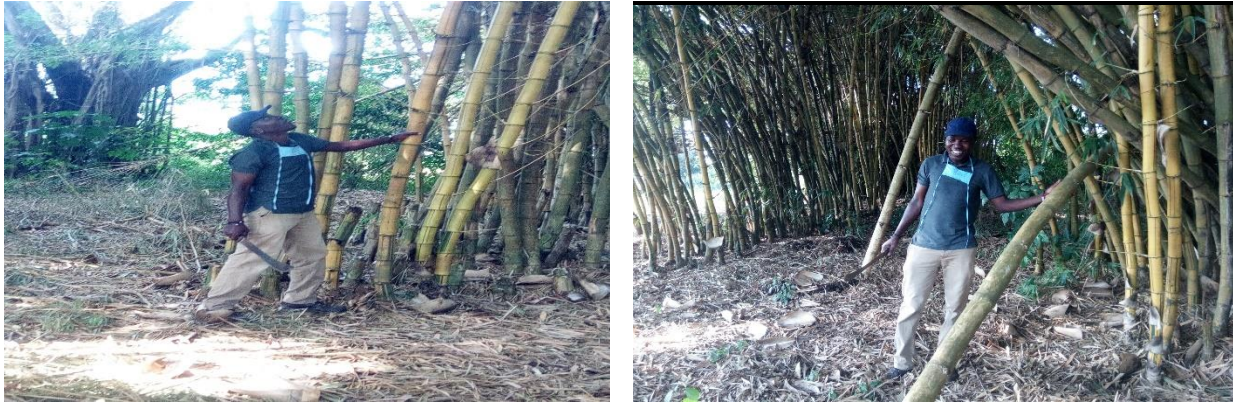
Figure.3.2 Left: Examining the Bamboo for Selection and Right: Cutting the bamboo samples at desired length for transportation to the Laboratory for the experiment.
