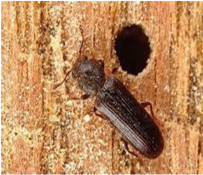
Figure 2.8: Bamboo culm bored by beetle.
