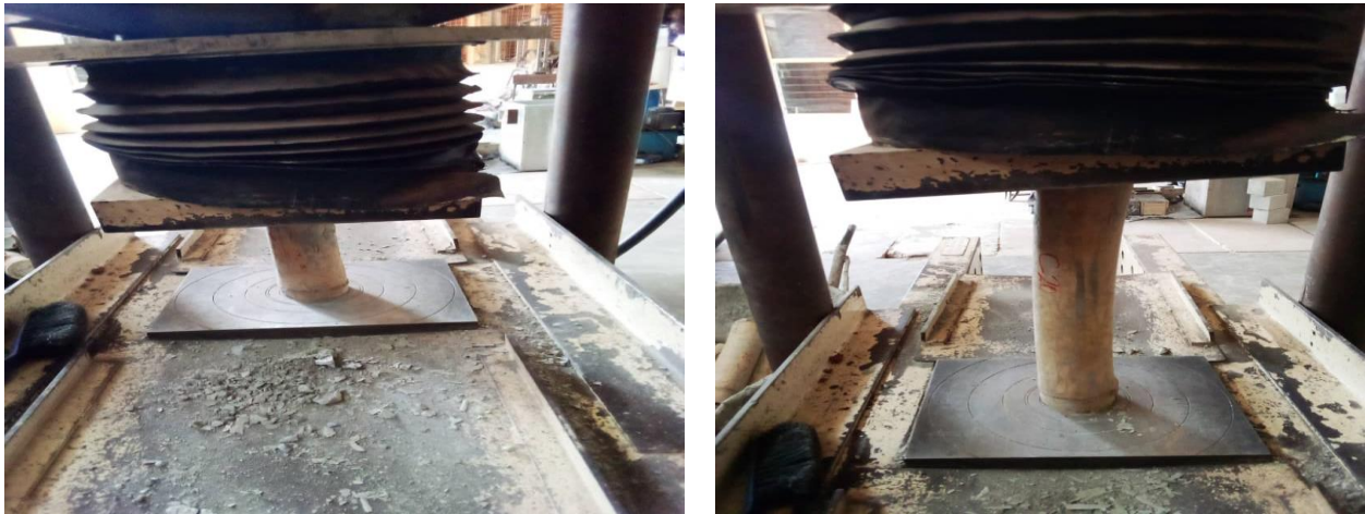
Figure 3.9: Conducting Compressive strength Test on the bamboo infilled concrete samples.
