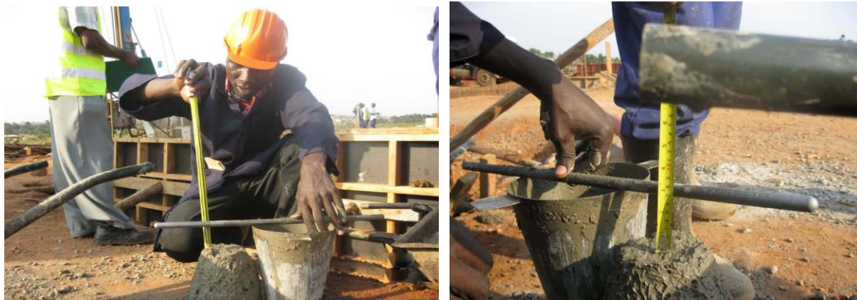
Figure 3.6: Performing slump tests for the concrete mix design.
