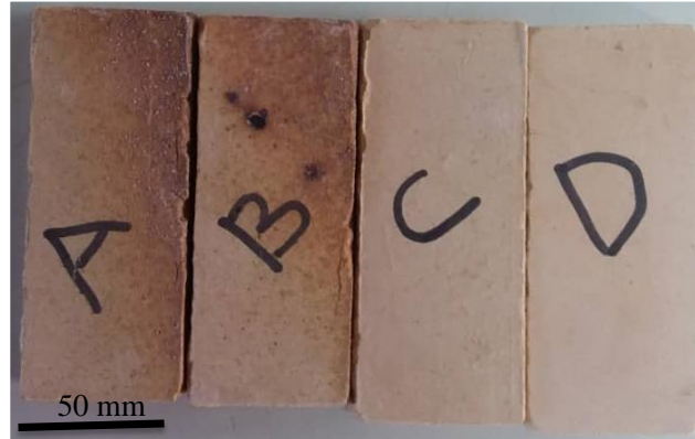
Figure 4.12: Optical image of tile samples A, B, C and D after firing whose mold dimensions were 110 mm × 50 mm × 10 mm.
