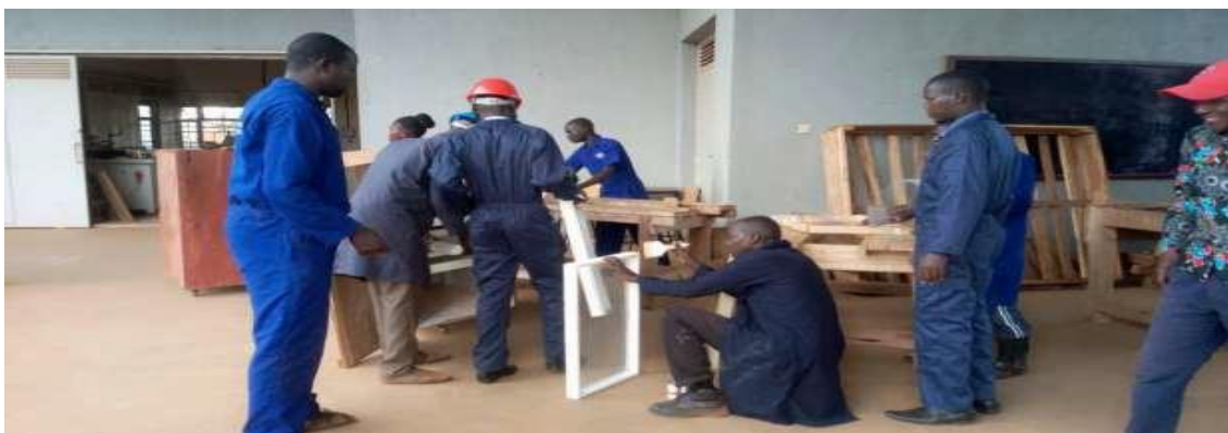
Figure 10: Trainees making drawers of the incubator
