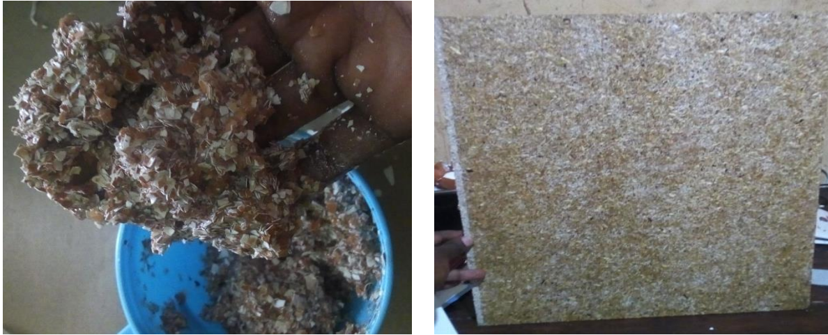
Figure 47 Mixing wood glue and making a flat surface
