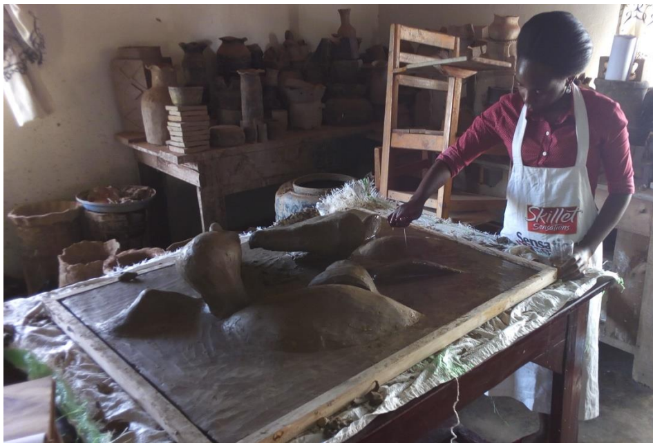
Figure 59 Adding oil to the clay work before the casting process
