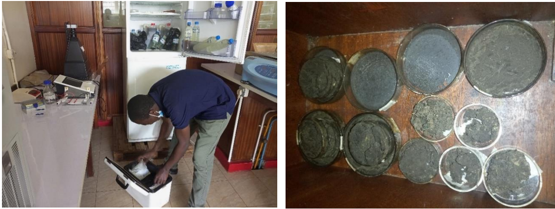
Figure 3. 8: Refrigeration of samples and determination of MC and TS
