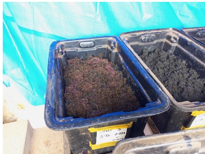
Figure 3. 3: Inoculating of sludge samples with earthworm densities during setup
