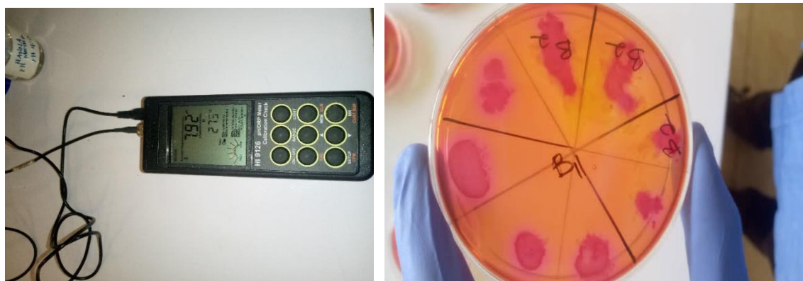
Figure 3. 9: pH - HANNAH instrument and a Completed Coliform Test (CCT)
