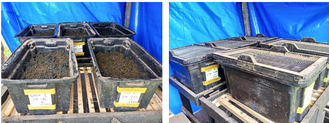
Figure 3. 7: Experimental setups for vermicomposting of sewage sludge at MAURIK
