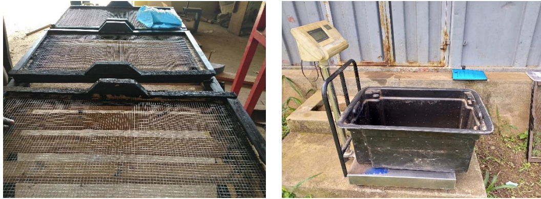
Figure 3. 4: Fabrication and weighting of compost bins for the setup
