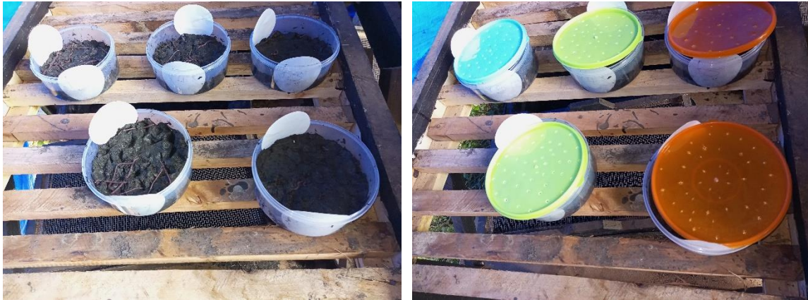
Figure 3. 6: Setup of the acute toxicity test for sewage sludge vermicomposting
