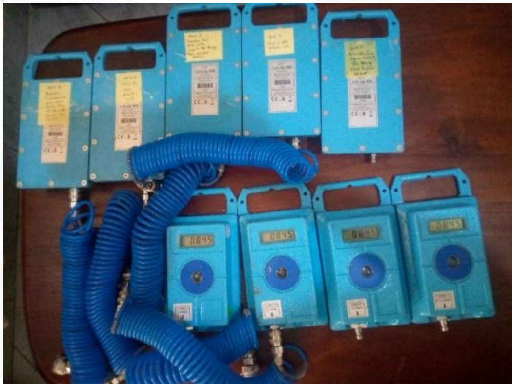
Figure 3.2: water pressure Loggers that was used to measure pressure in the water supply network
