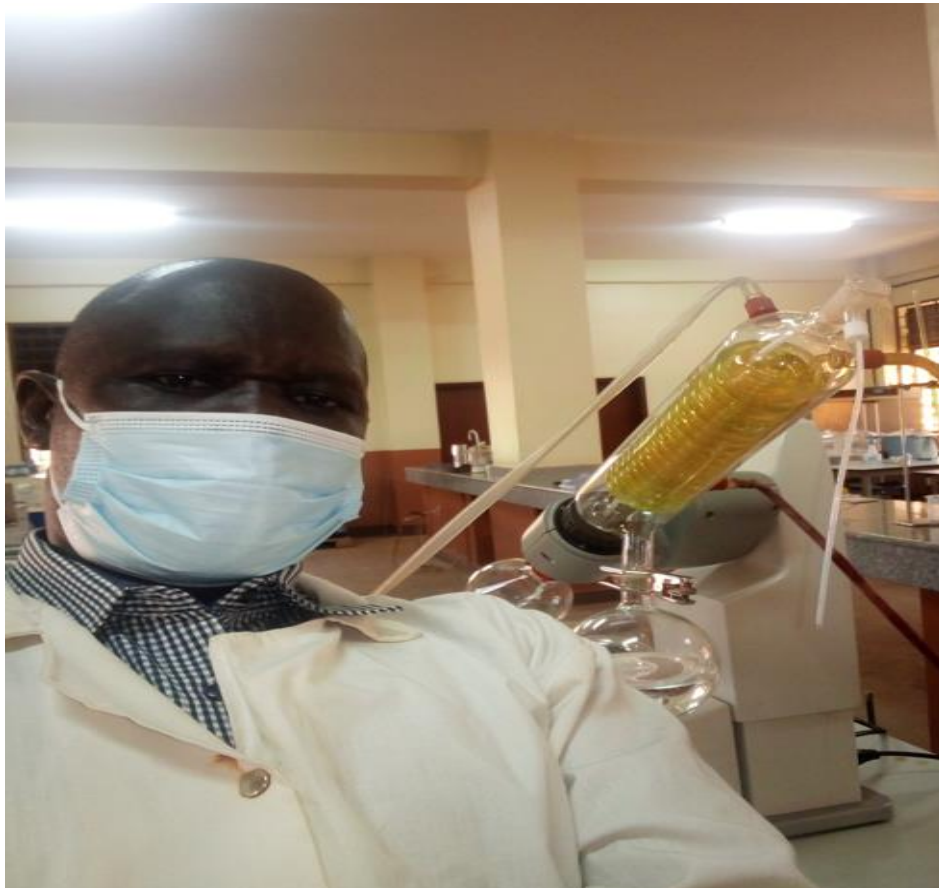
Concentration of the fractions collected using a rotary evaporator under reduced pressure.
