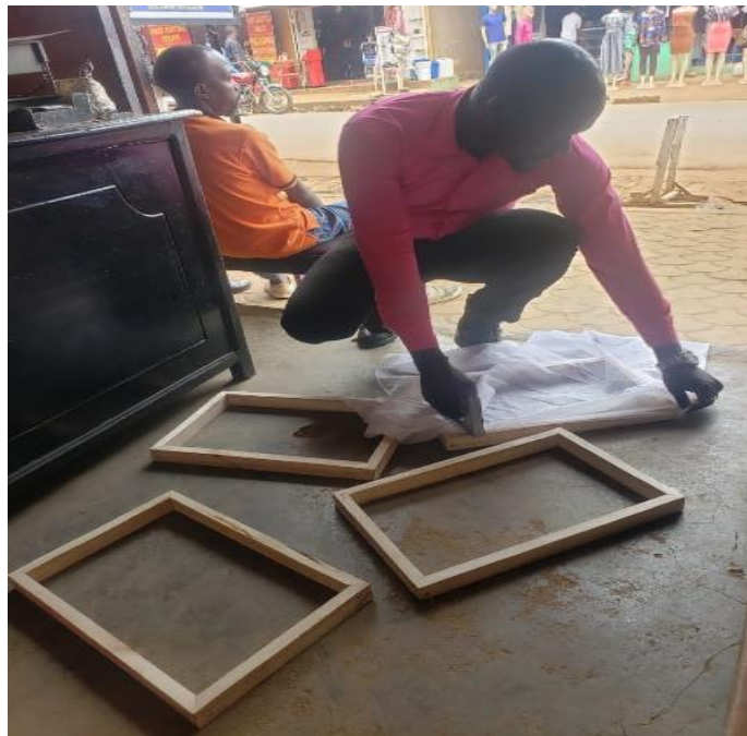
Plate 65: Researcher organising the already made frames and staples are being driven on to the net and them to the wood as shown. Source: Researcher, 2021
