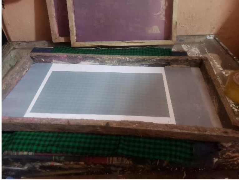
Plate 25: Screen is placed on top of the window on the Manyatta bedsheet ready for printing. (Source: Researcher, 2021)
