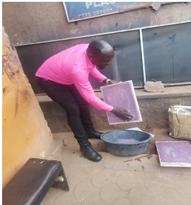
Plate 91: Researcher washing away the screen to remove unwanted paste so that it is clean for the next printing exercise. Source: Researcher, 2021
