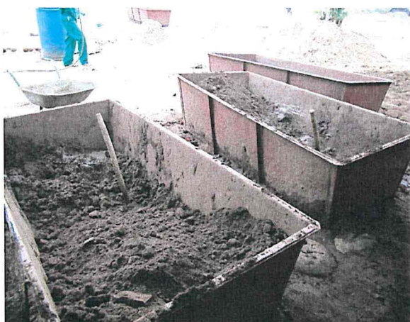
(a) Tools used for mixing motor at one of the TVET Centers in Juba (b) Tools used for mixing motor at one the workplaces in Juba
