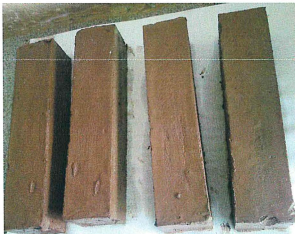
Figure 4.4 Slip casted brick samples
