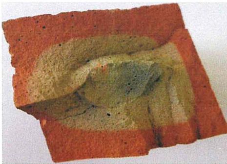
Figure 4.12: Pores in a thick fired brick sample
