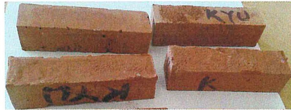
Figure 4.11 Slip casted fired brick samples
