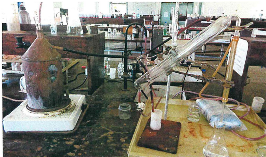
Figure 3.8: Distillation unit to distill off the Nitrogen
