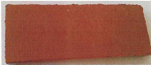
Figure 4.10 Wet pressed fired brick sample
