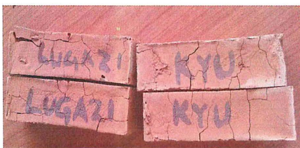
Figure 4.7 Slip casted fired brick samples
