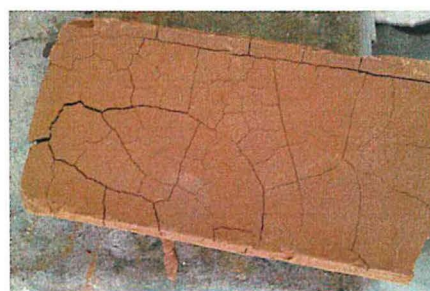
Figure 4.8 Wet compressed fired brick sample
