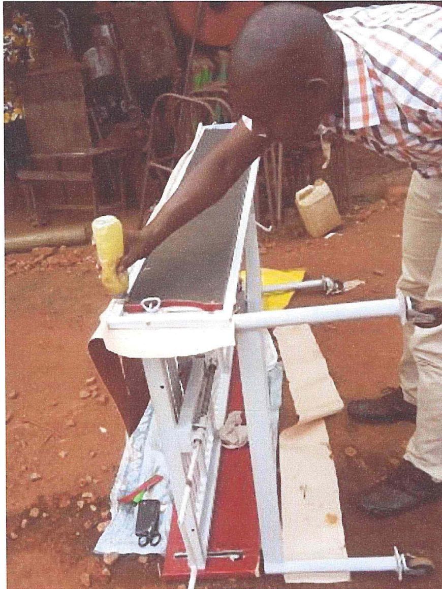
Figure 4.5.14: Turf adhesive being applied on Synthetic rubber, safety rail frame and synthetic leather prior bonding them together Source: Photograph by the Researcher, 2018
