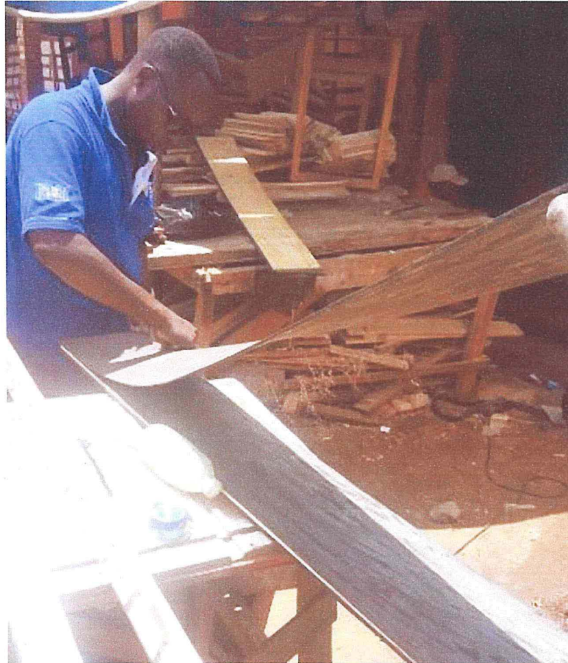
Figure 4.5.11: Synthetic rubber being cut to size and glued to the ply. Source: Photograph by the Researcher, 2018
