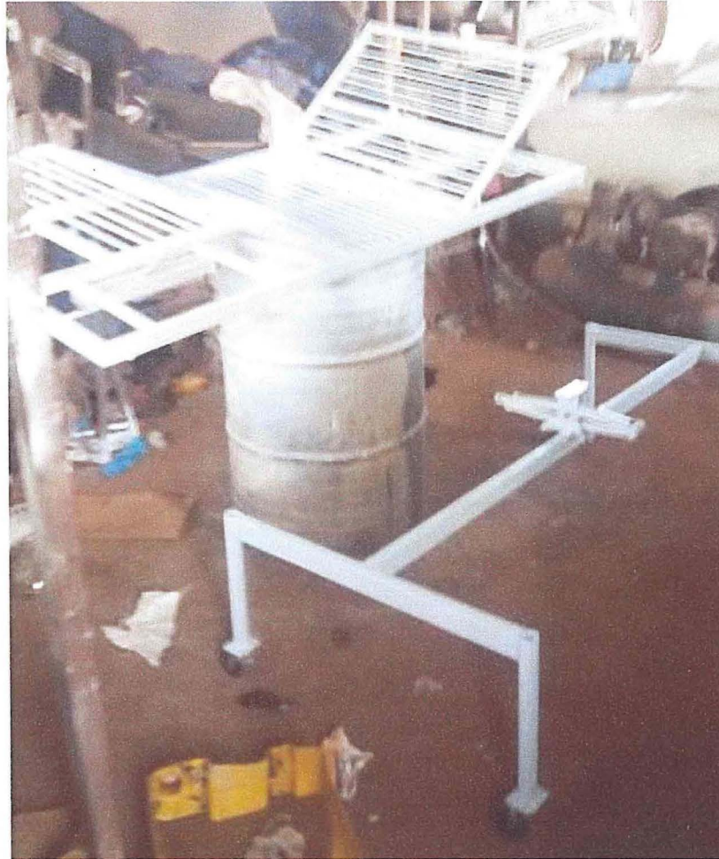
Figure 4.5.8 Stands and adjustment leg, thigh and back rests frame. Source: Photograph by the Researcher, 2018
