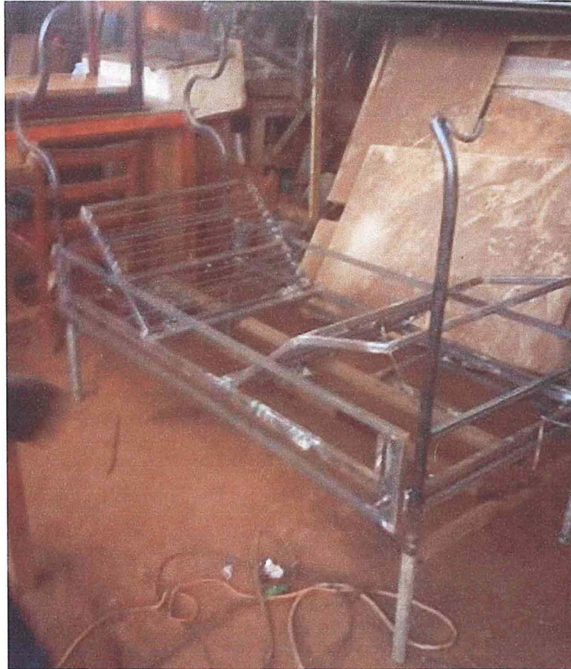
Figure 4.5.7 Stands and adjustment leg, thigh and back rests frame. Source: Photograph by the Researcher, 2018
