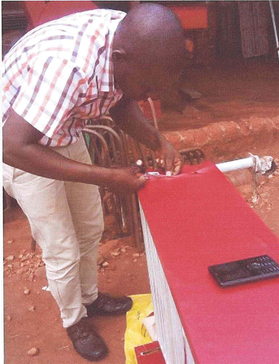
Figure 4.5.15 Finishing safety rails, hind and front upper stand sections with leather Source: Photograph by the Researcher, 2018
