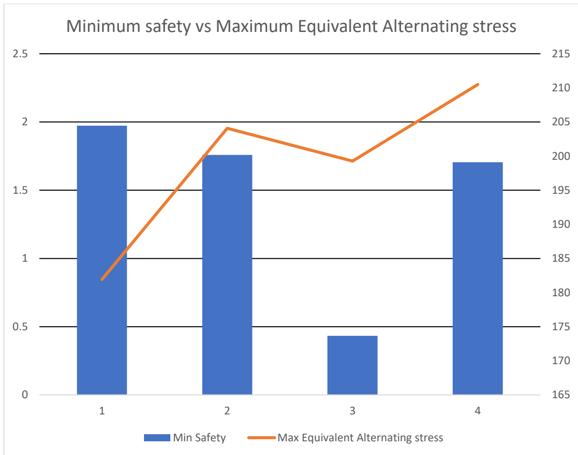
Figure 4.32: Minimum safety vs maximum Equivalent alternating stress
