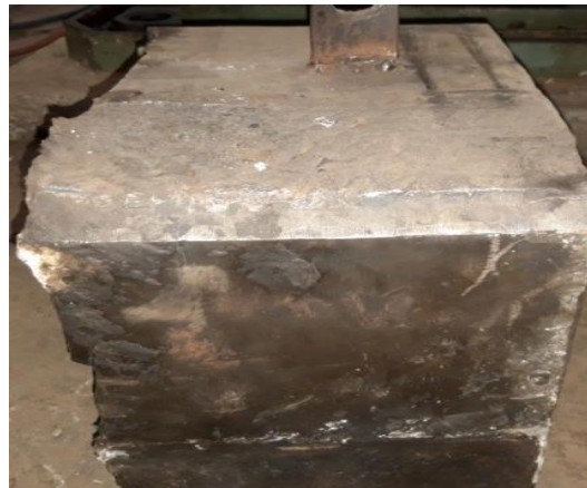
Figure 3.5: Specimen 3 cut from the broken square end for top roller shaft KE-8 in 4th Mill
