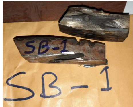
Figure 3.4: Specimen 2 cut from broken top roller SB-1 in 3rd mill
