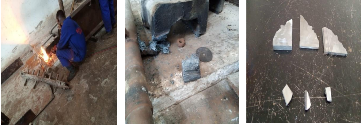
Figure 3.6: Specimen 4 cut from a worn box coupling for the top roller mill 4
