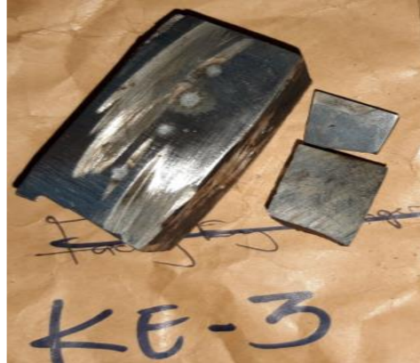
Figure 3.3: Specimen 1 cut from a failed top roller shaft KE-3 in 4th mill
