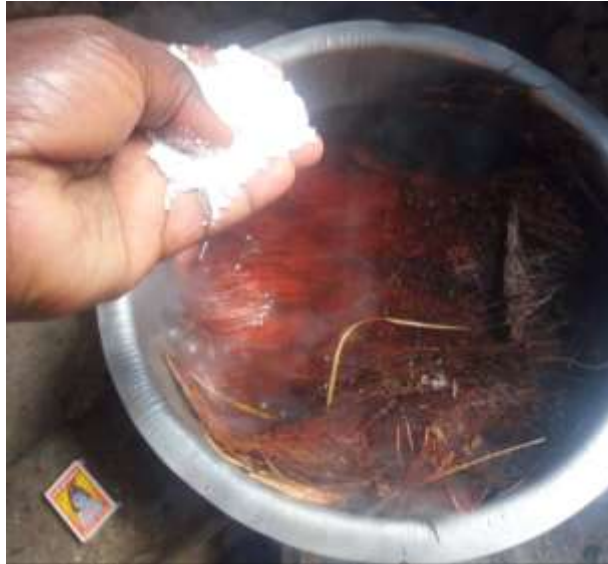
Figure 4.7: Boiling the date palm fibre in water mixed with salt Photo by: Researcher
