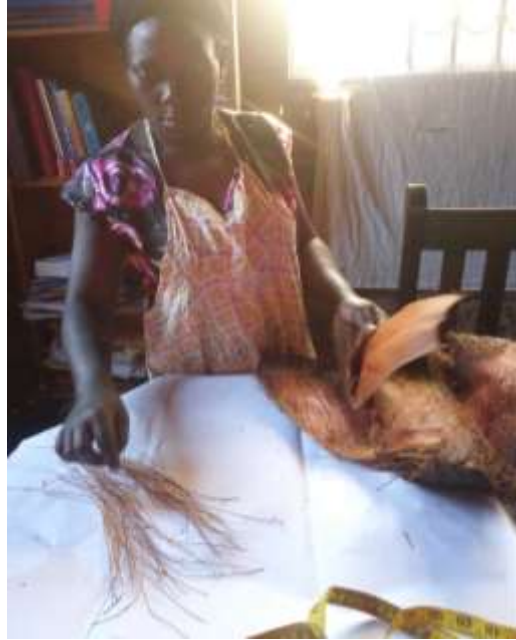
Figure 4.8 date- palm fibres being pulled out from the boiled date- palm fibres.
