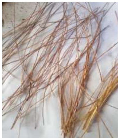
Figure 4.9: Stripes of date palm fibres removed from the boiled fibres.
