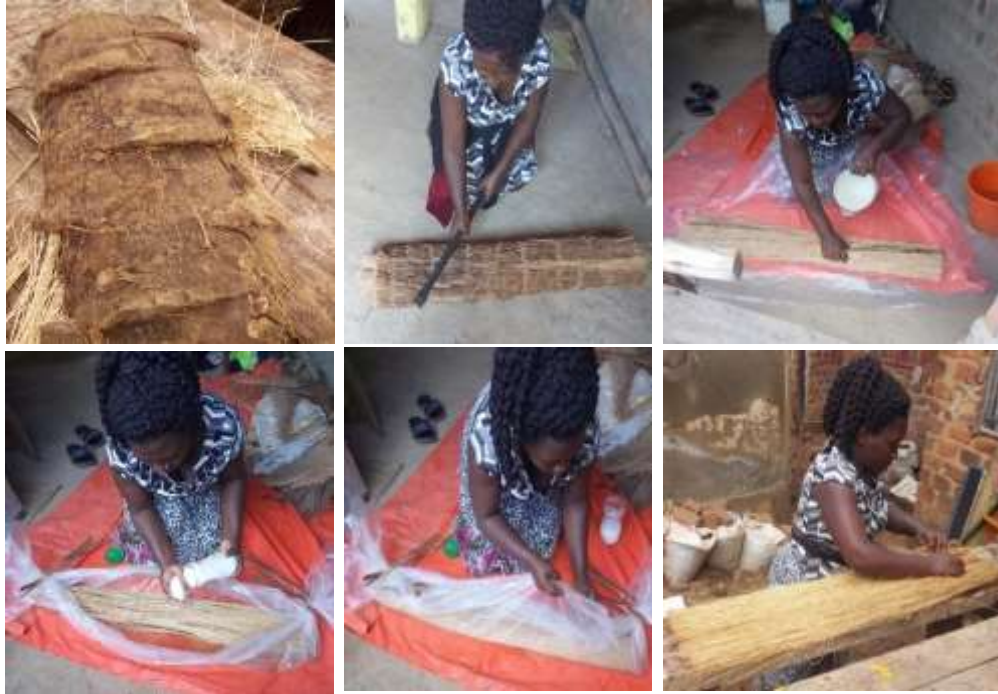
Figure 4.16 the process of extracting and socking the date- palm tree fibres in a mixture of salt and water.
