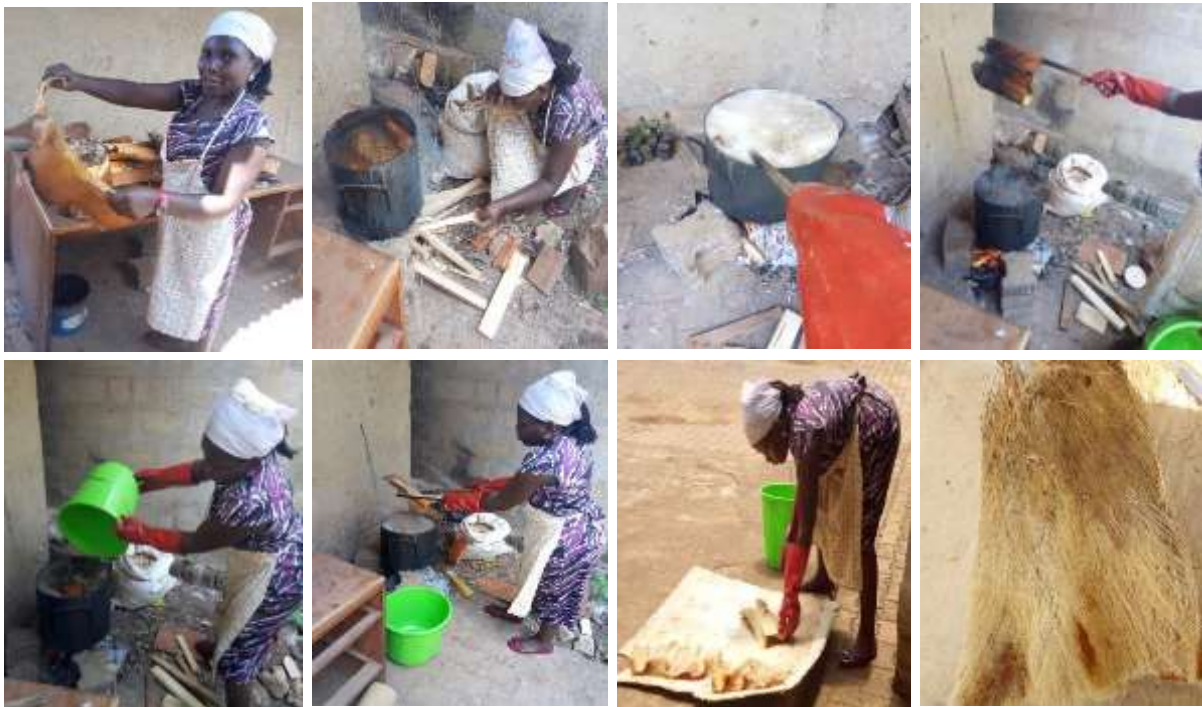
Figure 4.5 the process of boiling date- palm fibre in hydrogen peroxide. Photo by: Researcher
