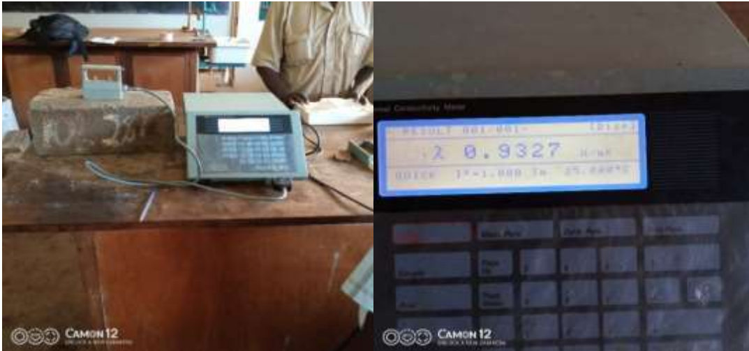
Figure 3-7: Determination of thermal conductivity of the blocks in the laboratory.
