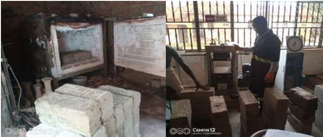
Figure 3-8: Firing and determination of residual compressive strength of blocks
