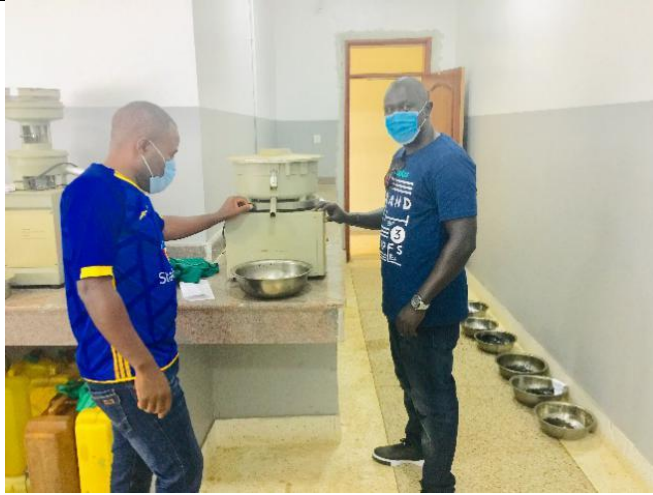
Extraction of cores to separate bitumen from aggregates
