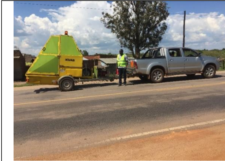
FWD testing at Km 97+700
