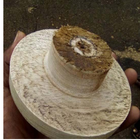
Poorly made the pattern
