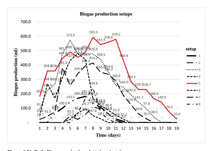
Figure 4-21: Daily Biogas production plotted against time
