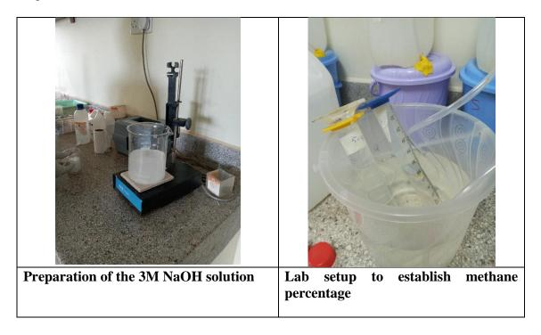
Figure 3-7: Establishment of methane concentration
