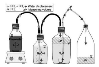
Figure 2-5: A biogas set up to determine methane concentration (Source: (Arthur, 2013)
