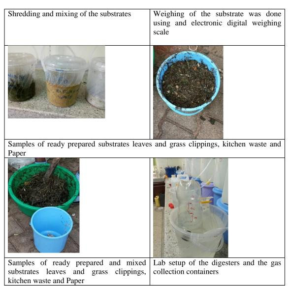
Figure 3-6: Preparation of substrates and laboratory setup
