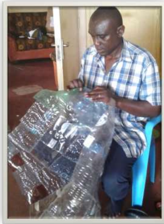
Figure 10: Patching flattened plastics
