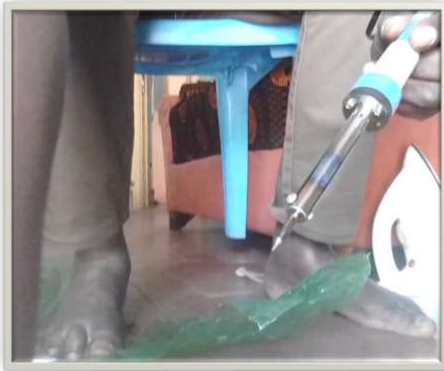
Figure 9: Piercing flattened plastic bottle using a soldering iron
