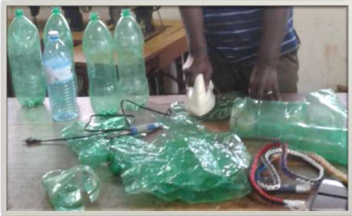
Figure 8: Ironing of plastic bottle cuts
